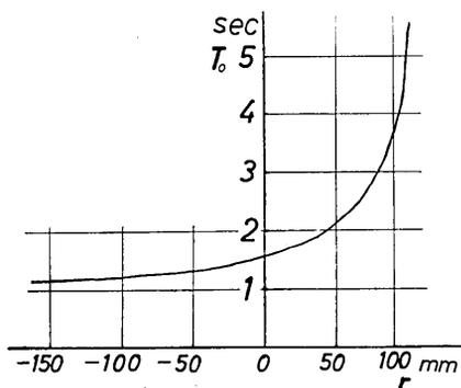
Fig. 10. Relationship between  $r$  and  $T_0 \left( = \frac{2\pi}{\omega_0} \right)$ .
