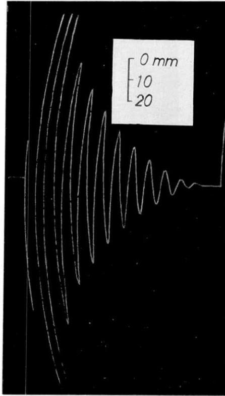
Fig. 15. Record of pendulum motion when  $r = 65.1 \text{ mm}$ ,  $T_0 = 2.48 \text{ s}$ ,  $x_f = 47 \text{ mm}$ ,  $A = 1.5 \text{ mm}$ ,  $\frac{\omega}{2\pi} = 100 \text{ c/s}$ .
