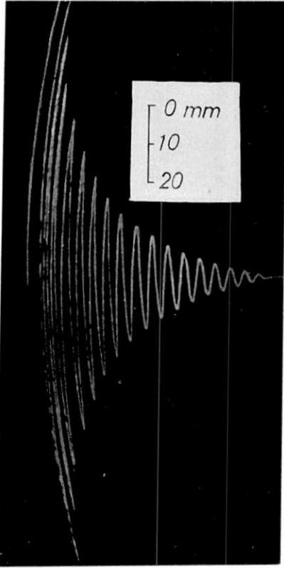
Fig. 14. Record of pendulum motion when  $r = -30.2 \text{ mm}$ ,  $T_0 = 1.40 \text{ s}$ ,  $x_f = 9.4 \text{ mm}$ ,  $A = 1.5 \text{ mm}$ ,  $\frac{\omega}{2\pi} = 100 \text{ c/s}$ .
