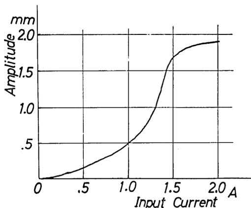
Fig. 12. Relationship between input exciting current and amplitude of vibration.
