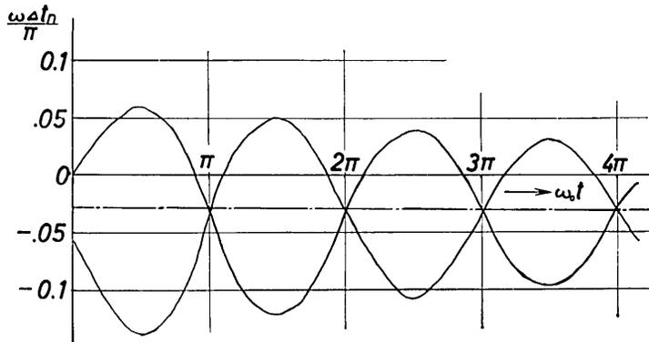
Fig. 7. Variation of  $\omega \Delta t_n$  when  $x_0=1$ ,  $x_f=0.5$ ,  $A=1$ ,  $\omega_0=1$ ,  $\omega=3$ ,  $h=\frac{1}{6\pi}$ .
