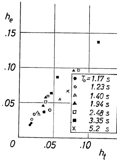
Fig. 17 (b). Relationship between  $h_e$  and  $h_t$  when  $f=100c/s$ .
