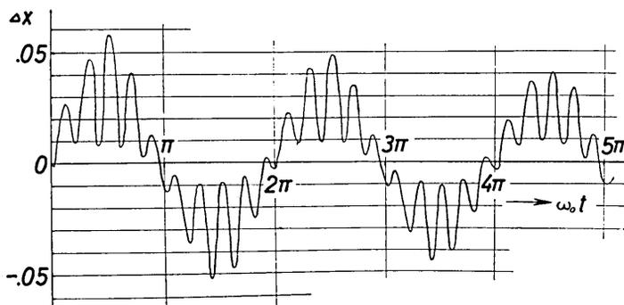
Fig. 3.  $\Delta x = x - x_0 \cos \omega_0 t e^{-h\omega_0 t}$  when  $x_0=1$ ,  $x_f=0.5$ ,  $A=0.5$ ,  $\omega_0=1$ ,  $\omega=10$ ,  $h = \frac{0.1}{\pi}$ .
