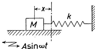
Fig. 1. Model of vibration system.
