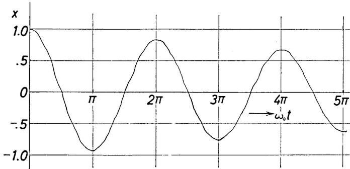
Fig. 2. Variation of  $x$  when  $x_0=1$ ,  $x_f=0.5$ ,  $A=0.5$ ,  $\omega_0=1$ ,  $\omega=10$ ,  $h=\frac{0.1}{\pi}$ .
