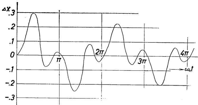
Fig. 6.  $\Delta x = x - x_0 \cos \omega_0 t e^{-h\omega_0 t}$  when  $x_0=1$ ,  $x_f=0.5$ ,  $A=1$ ,  $\omega_0=1$ ,  $\omega=3$ ,  $h=\frac{1}{6\pi}$ .
