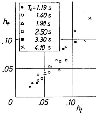
Fig. 17 (d). Relationship between  $h_e$  and  $h_t$  when  $f=316c/s$ .
