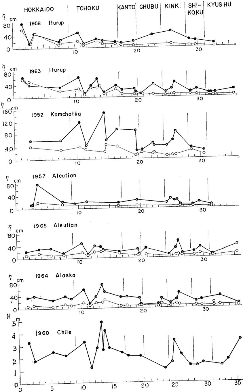
Fig. 3. Distribution of crest-height (above the ordinary tidal level) on the coast of Japan. Numerals on the abscissa correspond to the serial numbers in Fig. 2.
