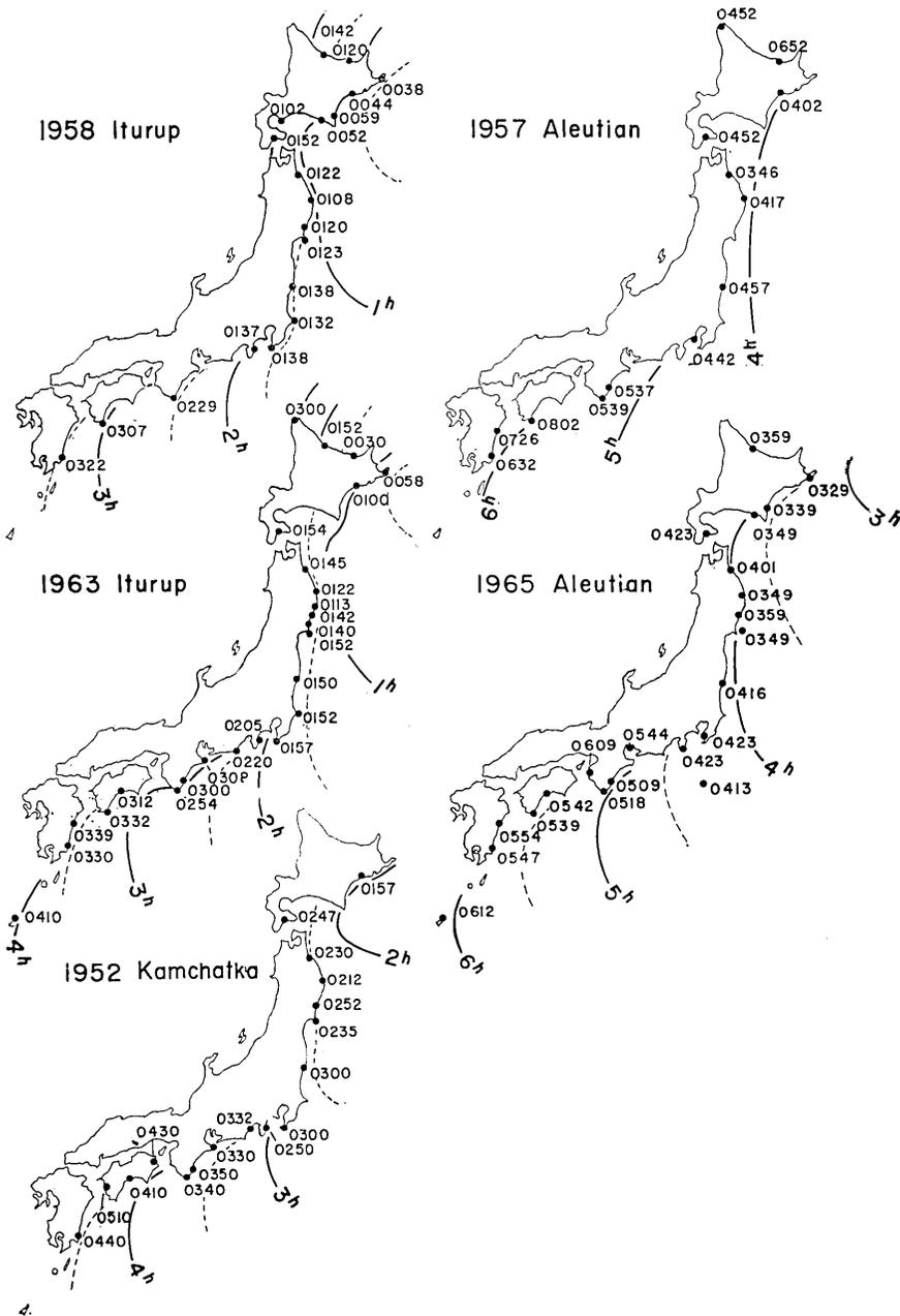
Fig. 6(a). Refraction diagrams obtained from the arrival times of wave fronts. Arabic numerals indicate travel time (h, m).
