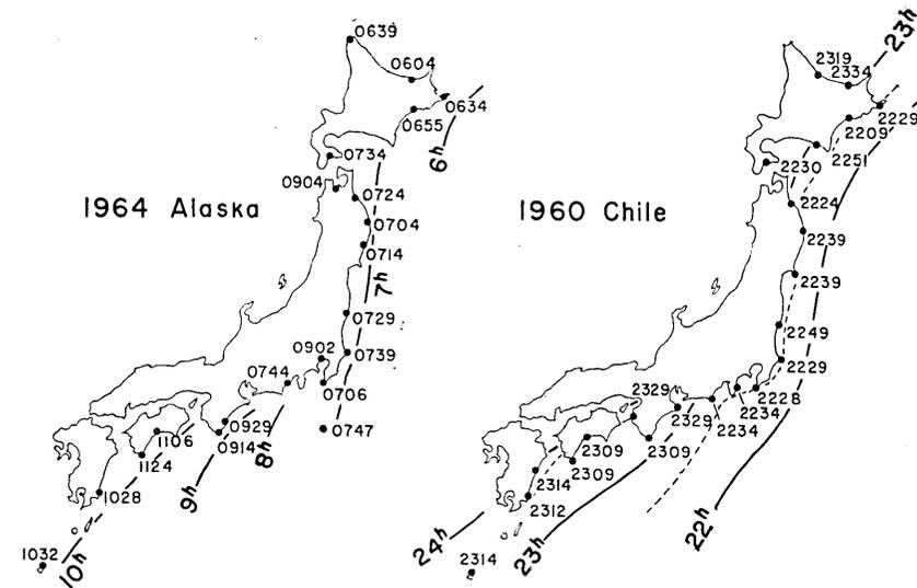
Fig. 6(b). Refraction diagrams for the cases of the 1964 Alaska and the 1960 Chilean tsunamis.
