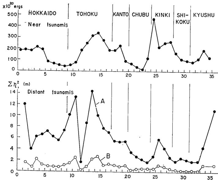
Fig. 5. Comparison of distribution of tsunami energy on the coast of Japan between the near tsunamis and the distant tsunamis.
