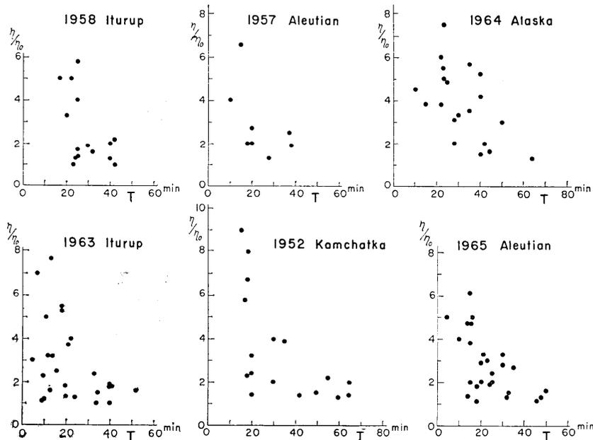
Fig. 4. The relation between crest-height ratios ( $\eta$ : Maximum wave,  $\eta_0$ : Initial wave) and period of the maximum wave.
