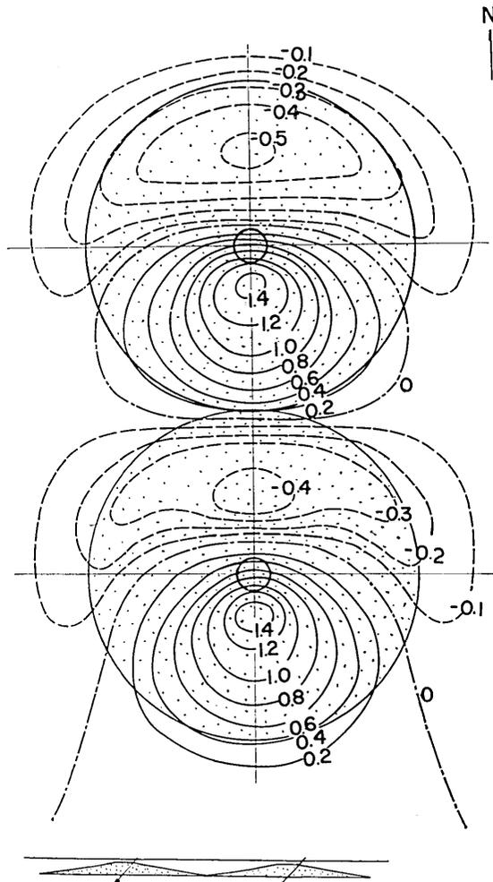
Fig. 9.  $\Delta F$  over two cones closely placed. The line connecting the centres runs in a north-south direction. The parameters of the cones and the relation between the magnetization and the geomagnetic field are the same as those for Fig. 2.
