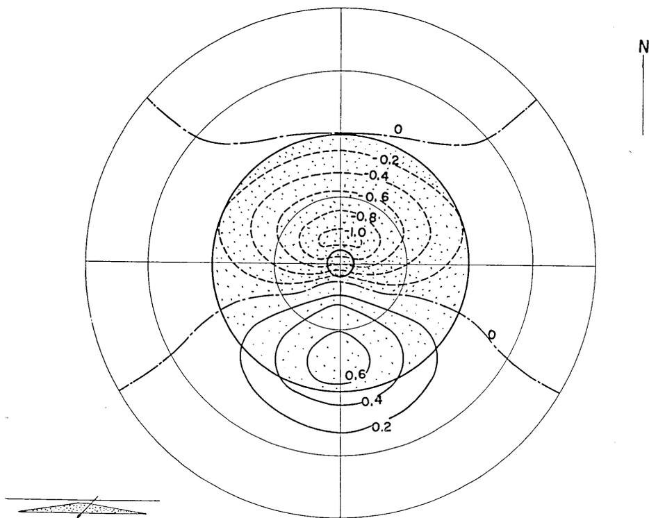
Fig. 2a.  $\Delta X$  over a magnetized circular cone, which is shown by the shaded circle, at a height of 0.2 in units of the bottom radius. The numerals indicate the field intensity when the intensity of magnetization and the bottom radius are taken as unity. It is assumed that the direction of magnetization lies in the magnetic meridian plane and that its inclination agrees with the geomagnetic dip which is taken as  $48^\circ$ . The slope angle is assumed as  $10^\circ$ .
