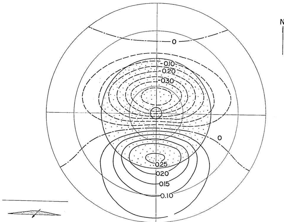
Fig. 4a.  $\Delta X$  over a cone of which all the parameters are the same as those for Fig. 2. The flight height is 0.5.
