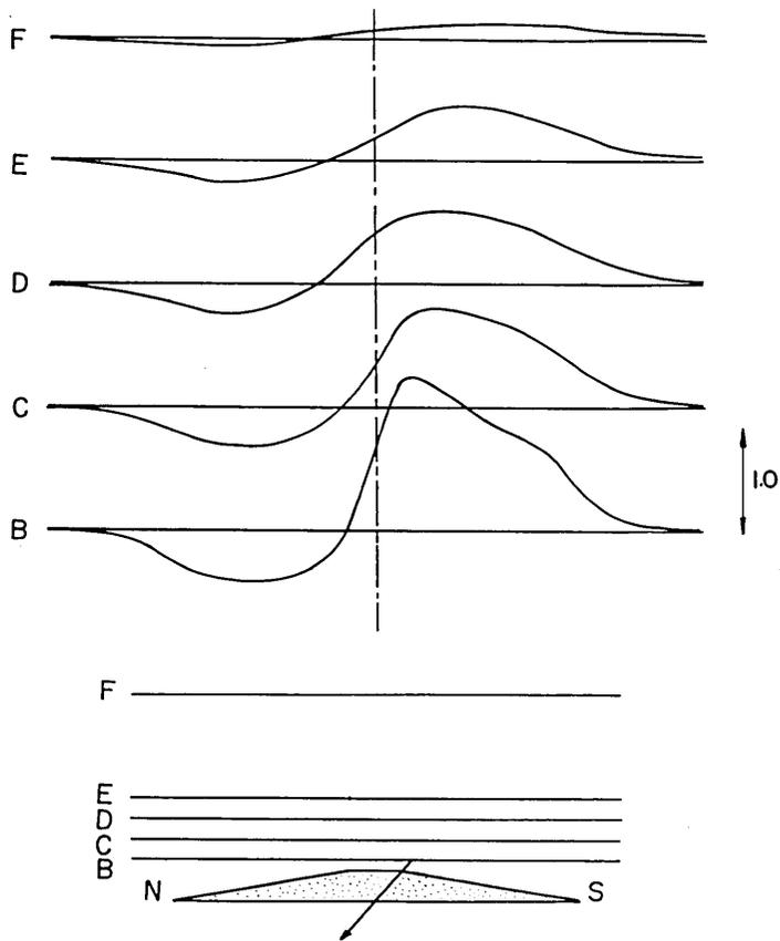
Fig. 7.  $\Delta F$  profiles similar to Fig. 6. The slope angle is  $10^\circ$ . The flight heights are taken as 0.2, 0.3, 0.4, 0.5 and 1.0.
