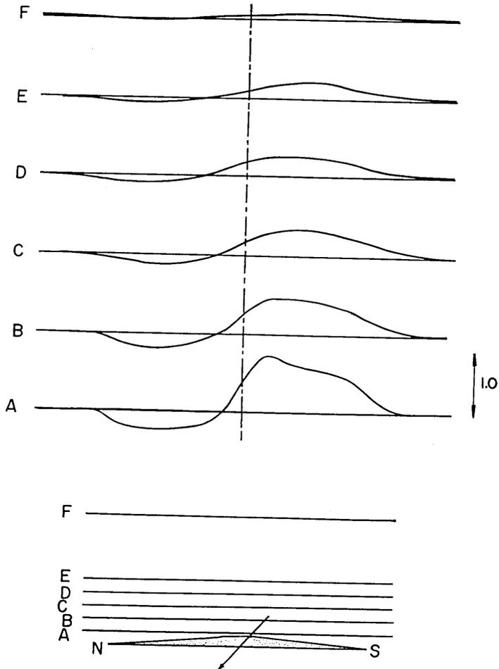
Fig. 6.  $\Delta F$  profiles along the north-south line passing through the centre of a cone of which the slope angle is  $5^\circ$ . The direction of magnetization and its relation to the geomagnetic field have been given in the caption of Fig. 2. The intensity of magnetization and the bottom radius are both taken as unity. The flight heights are taken as 0.1, 0.2, 0.3, 0.4, 0.5 and 1.0.
