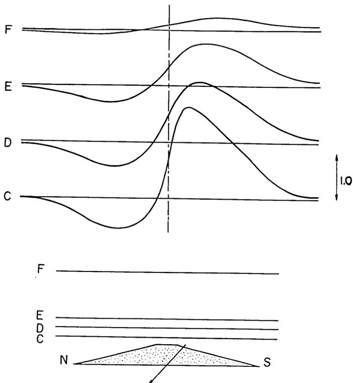
Fig. 8.  $\Delta F$  profiles similar to Fig. 6. The slope angle is  $15^\circ$ . The flight heights are taken as 0.3, 0.4, 0.5 and 1.0.
