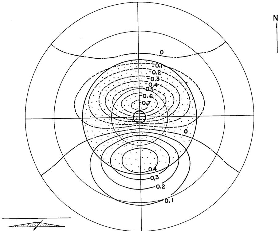
Fig. 3a.  $\Delta X$  over a cone of which all the parameters are the same as those for Fig. 2. The flight height is 0.3.
