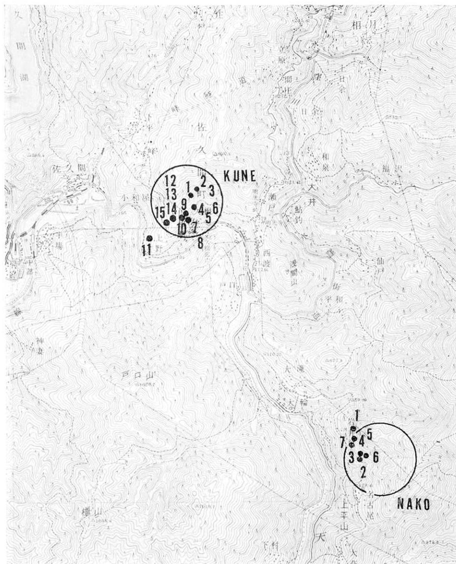
Fig. 12. Localities of boreholes in Kune (Honzan) and Nako Mines. Numbers to the circles refer to those in Table 9. The map covers the area from  $35^{\circ}02' N$  to  $35^{\circ}07' N$  in latitude and from  $137^{\circ}48' E$  to  $137^{\circ}53' E$  in longitude.
