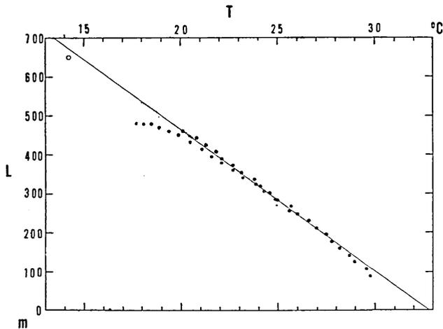
Fig. 9. Temperature-altitude relation in Kamioka Mine. Hollow circle at the upper left corner: Borehole B-4, Hollow circles: Borehole XH 78, Full circles: Borehole XH 94.
