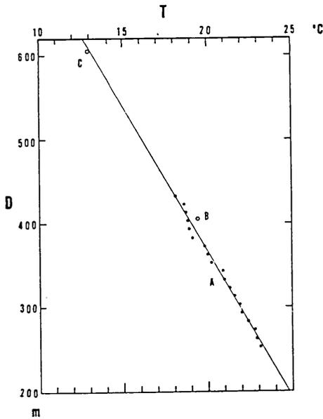
Fig. 11. Subterranean temperature vs. altitude in Nakatatsu Mine.
