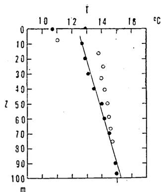
Fig. 16. Temperature depth relation in Minenosawa Mine. Full circles: Borehole No. 2. Hollow circles: Borehole No. 1, which was being drilled at the time of measurement.
