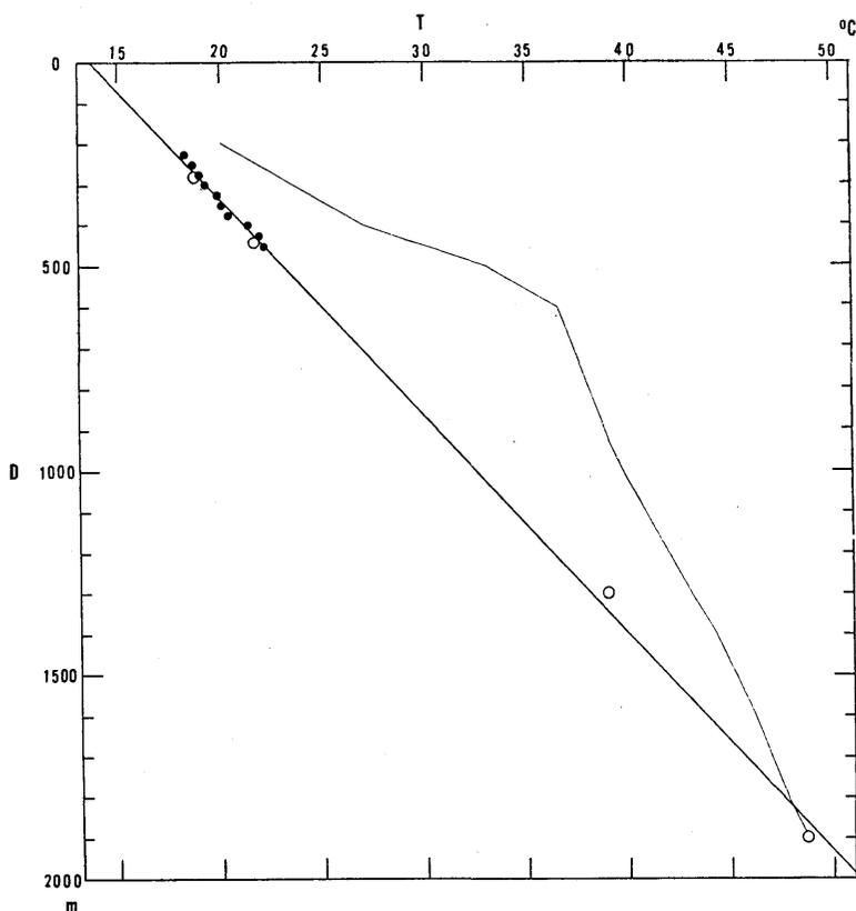
Fig. 3. Temperature—depth relation in Mobarra gas field.
