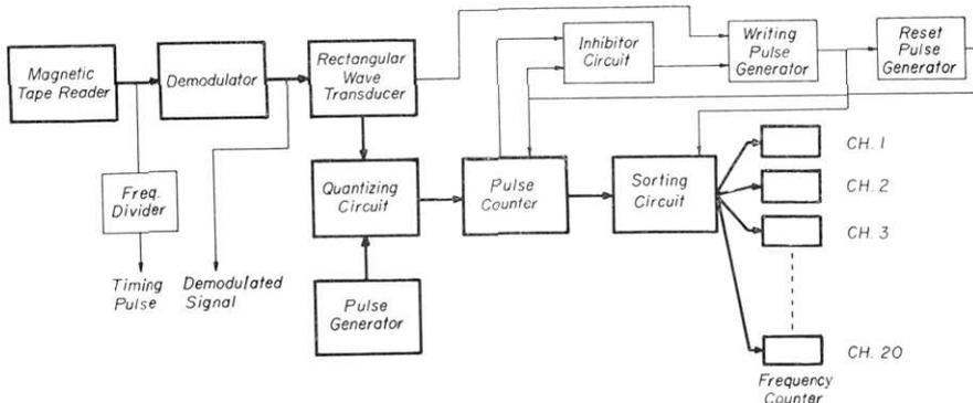
Fig. 4. Block diagram of period distribution analyser.
