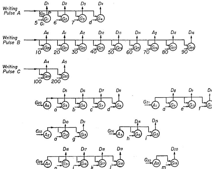
Fig. 7. Schematic diagram of the second sorting and writing circuits. G: Simultaneous gate (6BE6). A: Phase inverter (1/2 6J6). D: Dekatron (4CG-10A).
