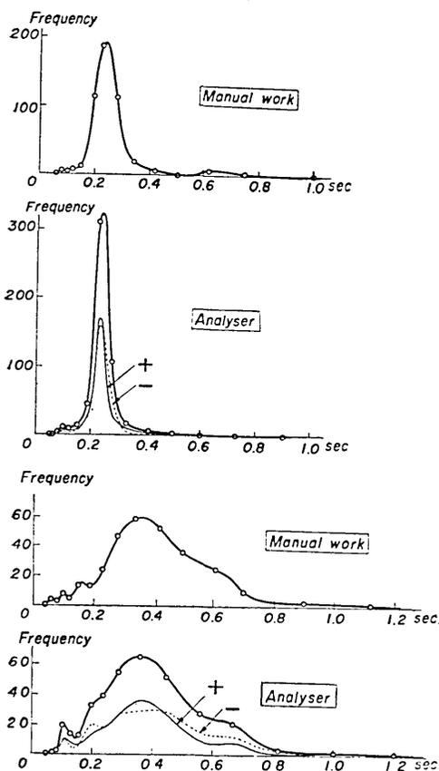
Fig. 8. Examples of frequency-period curves of microtremors analysed by the analyser and manual works.
