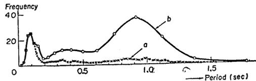
Fig. 1. Examples of frequency-period curves of microtremors obtained by different methods of classification. a; Constant period interval ( $\Delta T = 0.02$  sec). b; Constant period interval in the logarithmic scale ( $\alpha=0.2$ ).
