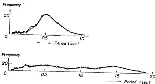
Fig. 2. Examples of frequency-period curves of microtremors obtained by the original (○) and modified (×) classification methods.
