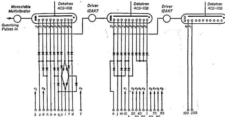
Fig. 6. Schematic diagram of the first sorting circuit.
