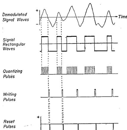
Fig. 5. Waveforms and phase relationship of signals used in the analyser.
