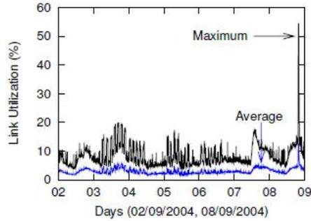
Figure 5.1: Maximum and average link utilization in the Abilene network
