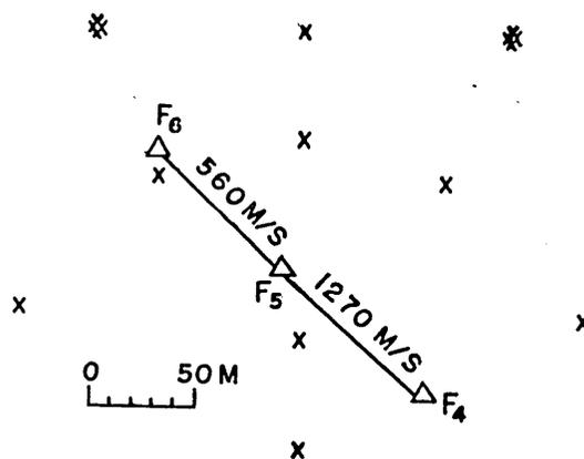
Fig. 11. Progress of a fracture in the ice-sheet.
