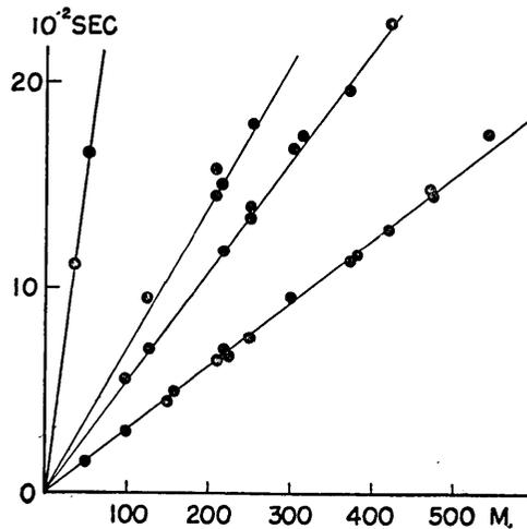
Fig. 6. Travel time curves for various event due to the detonation from the small charges measured on the ice.
