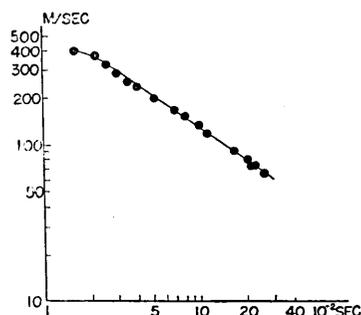
Fig. 8. Dispersion curve of flexural waves in the ice-sheet.
