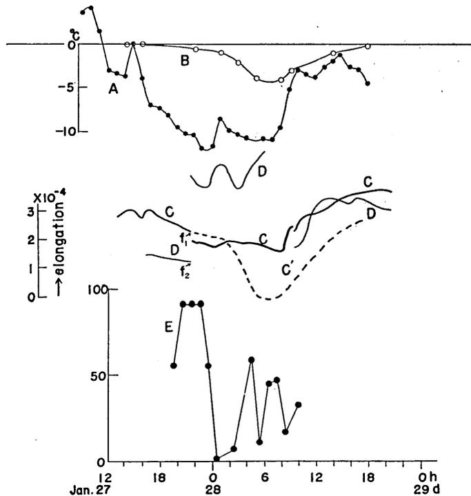
Fig. 4. An enlargement of part of the curves in Fig. 3, on Jan. 27 and 28. A is the air temperature, B is the temperature in the ice-sheet, C and D are records of extensometers and E is the frequency of ice tremors.
