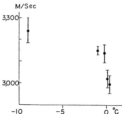
Fig. 7. Velocity of  $p$  waves in the ice versus air temperature.
