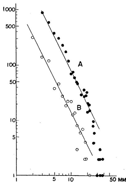
Fig. 5. Frequency distribution of maximum amplitude of the ice tremors. The data of the curve A are obtained from the detector installed at  $D_1$  in Fig. 9, and of curve B from  $D_2$ .
