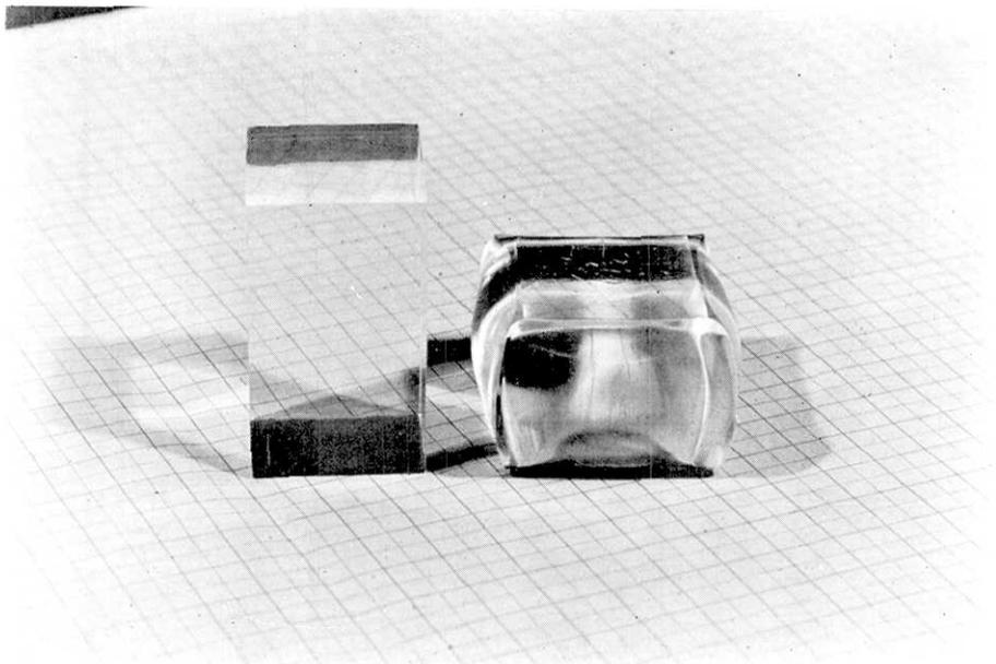
Fig. 14. Methyl-methacrylate specimen, original shape (left) and deformed one (right), respectively.
