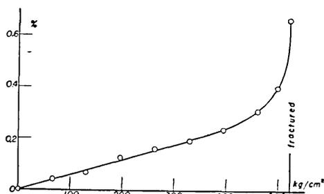
Fig. 6. Deformation curve of marble specimen.
