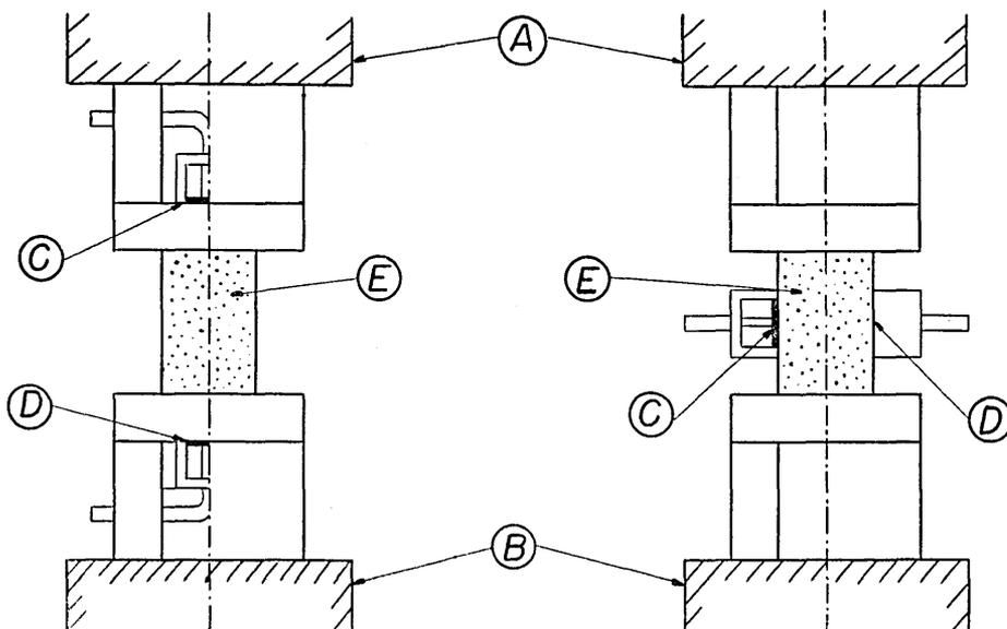
Fig. 1. Experimental arrangement for the determination of the velocity propagated parallel to the axis.
