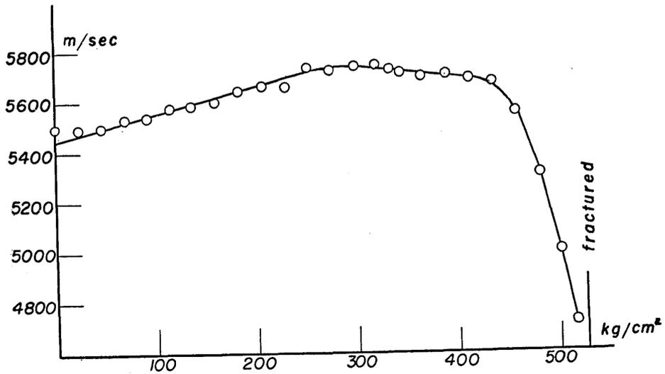
Fig. 3. Uniaxial pressure versus velocity of dilatational waves propagated along the axis of the pressure.
