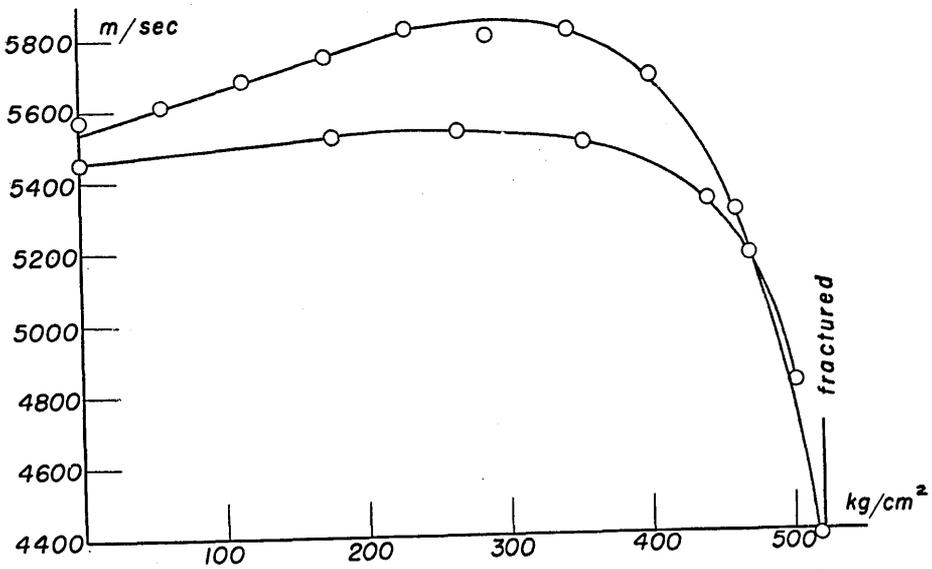
Fig. 4. Uniaxial pressure versus velocity of dilatational waves propagated parallel to the axis of the pressure.
