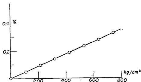
Fig. 7. Deformation curve of methyl-methacrylate specimen.
