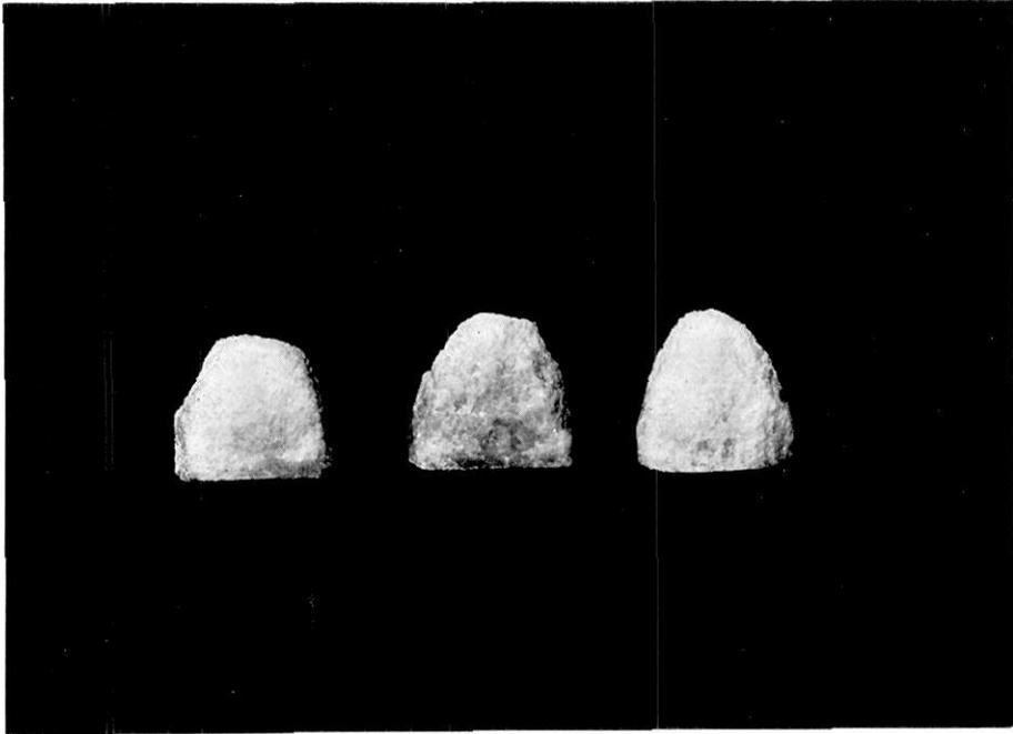
Fig. 13. Pyramids of marble specimen after fractured.
