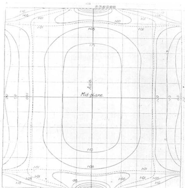
Fig. 9. Distribution of principal stress  $\hat{\sigma}$  inside the cylinder (case of compression between rough rigid plane) after Filon.
