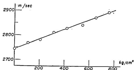
Fig. 5. Velocity of dilatational wave in methyl-methacrylate versus pressure.
