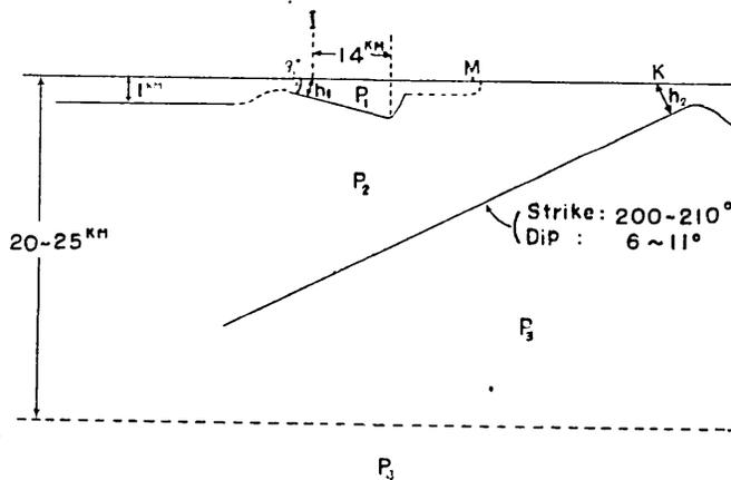
Fig. 1. Underground structure of the north-eastern part of Japan obtained by R. G. E. S.
