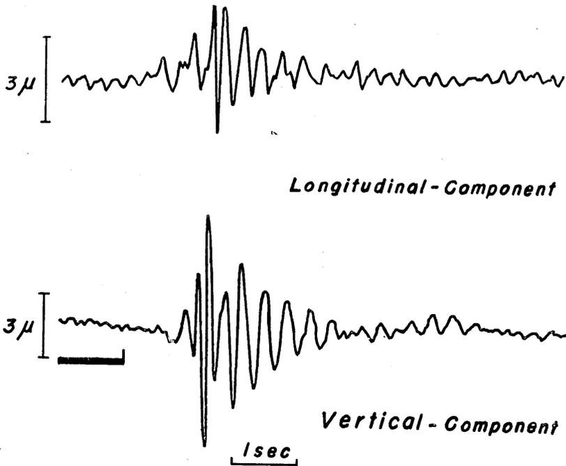
Fig. 3. Earth-vibration by falling of a mass recorded at 130 m distance.
