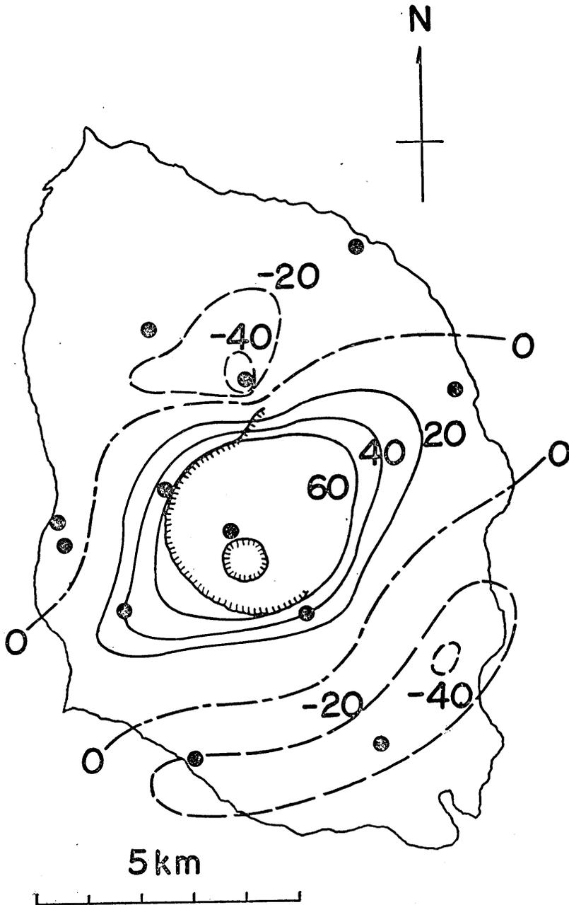
Fig. 6. The distribution of changes in vertical component. The unit is *gamma*.
