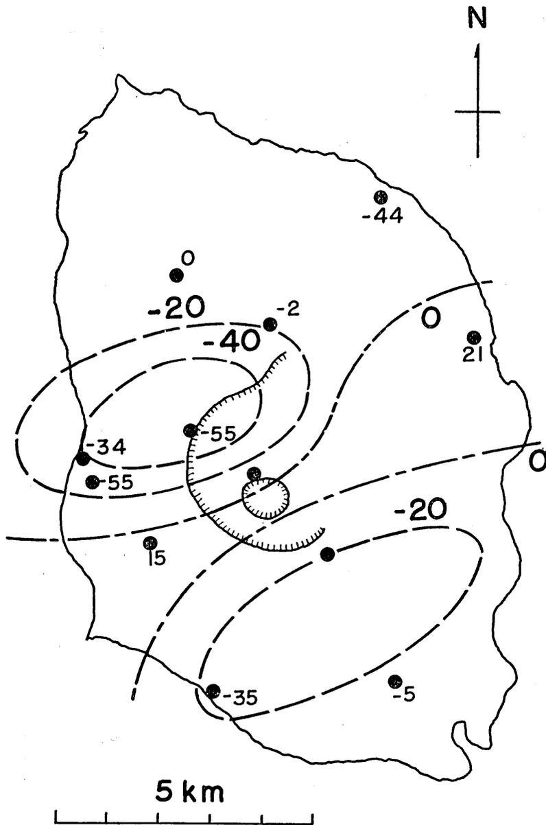
Fig. 4. The distribution of changes in geomagnetic north component. The unit is *gamma*.
