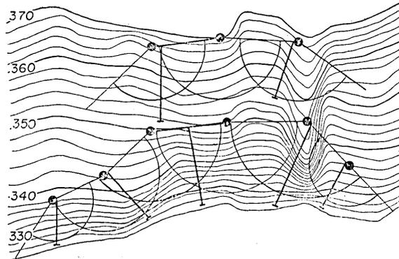
Fig. 2. Location plan of the explosive chambers and the area to be loosened by each chamber charge.
