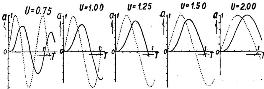
Fig. 9. The initial motion of the pendulum (solid line) caused by a sinusoidal torsional vibration (dotted line) suddenly applied to its head.
