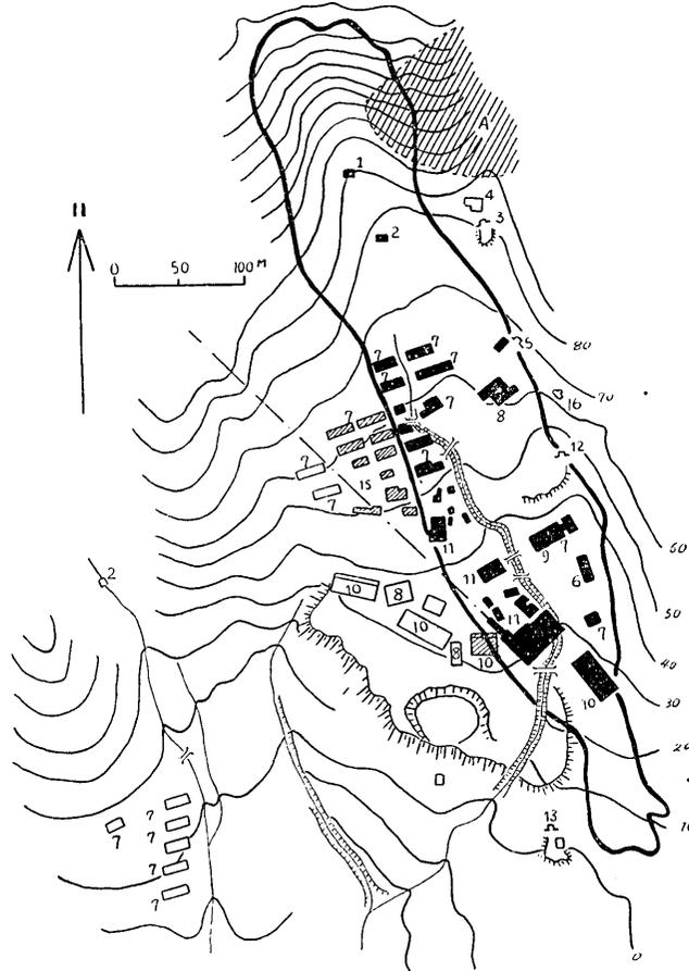
Fig. 5. Topography of the present land-slide. Contour lines drawn every 10 m. The thick closed curve in the figure gives an outline of the land-slide. Buildings painted black were destroyed; the hatched ones, burnt. The shaded area at the upper right corner shows the location of the ore deposit. A, the out-crop.
