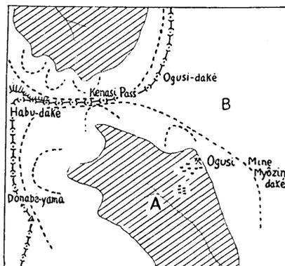
Fig. 4. Geological map of the mine and vicinity. Semi-circles in dotted line show the explosion craters.
