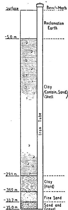
Fig. 3. Sectional view of the bore hole at Kazuya Primary School and B. M. S-1.
