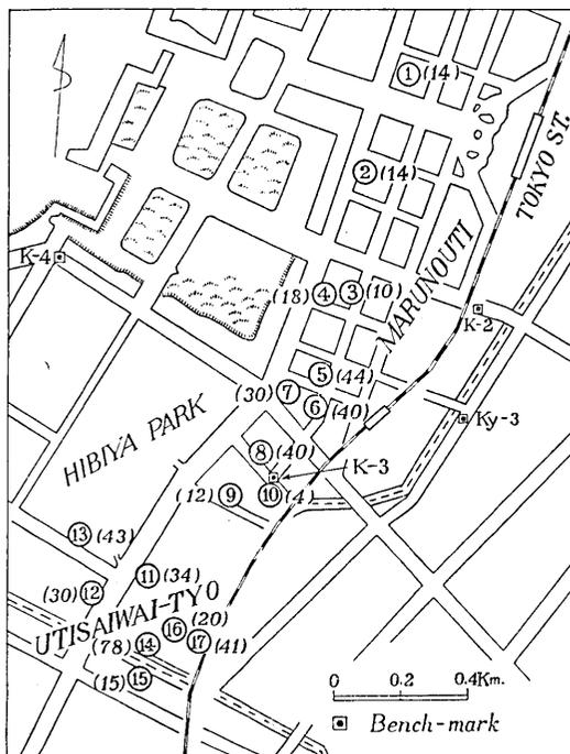
Fig. 2. Distribution of buildings, uprise of which being measured. (The bracketed numerals denote the amounts of uprise in cm)
