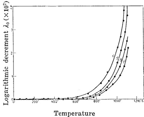
Fig. 7. Curves showing that the logarithmic decrements of the oscillations differ with different fibres at high temperature.
