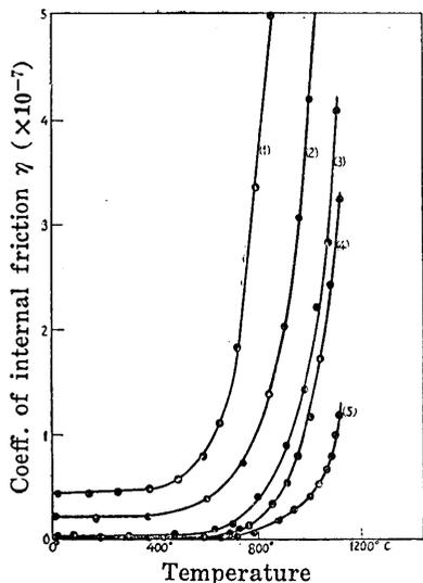
Fig. 9. Curves showing the relation between the coefficients of internal friction and temperature.
