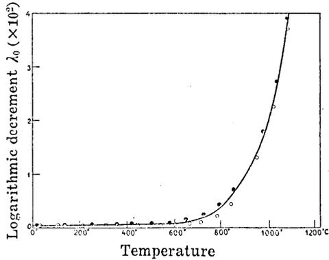
Fig. 6. Relation between observed logarithmic decrement  $\lambda_0$  of the oscillation and temperature.
