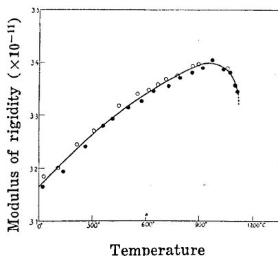
Fig. 4. Curve showing the change in rigidity of amorphous silica fibre with temperature.
