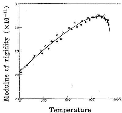
Fig. 5. Curve showing the change in rigidity of amorphous silica fibre with temperature.
