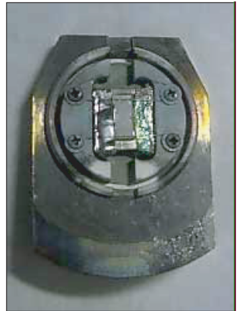
Figure 2.5: Sample holder used in film growth. Only the center part of the sample holder is actually heated.
