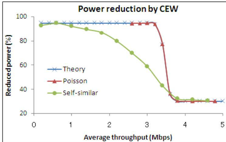
Figure 4.6: Simulation results on CEW ( Effect of average throughput)
