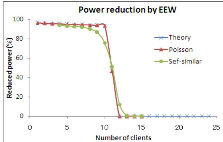
Figure 4.9: Simulation results on EEW ( Effect of number of clients)
