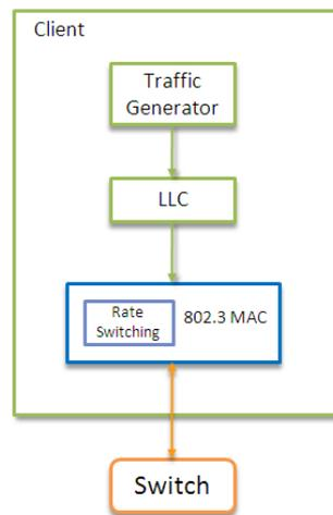
Figure 4.2: Simulator model for EEE
