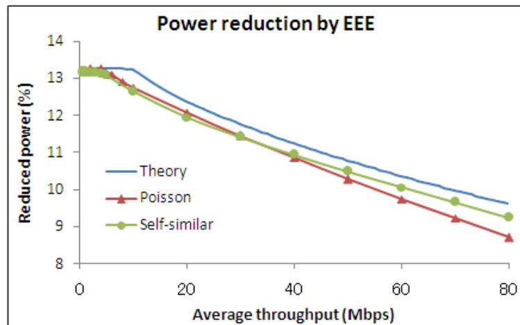
Figure 4.4: Simulation results on EEE ( Effect of average throughput)
