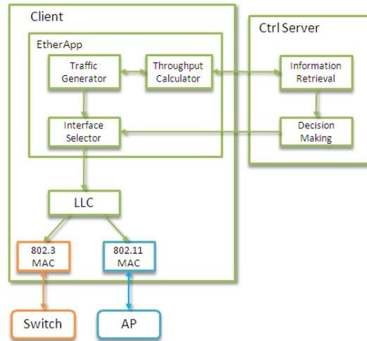
Figure 4.1: Simulator model for EEW
