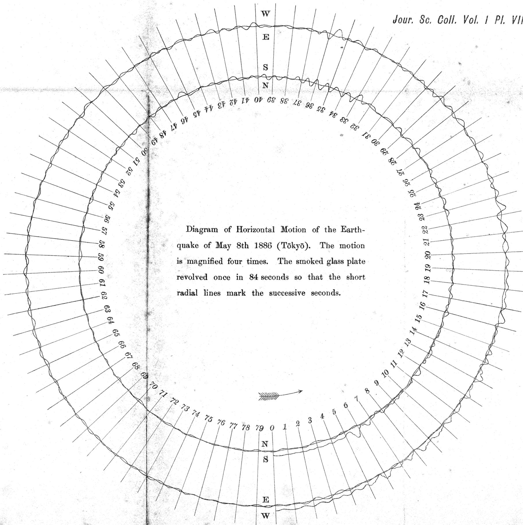
Diagram of Horizontal Motion of the Earthquake of May 8th 1886 (Tōkyō). The motion is magnified four times. The smoked glass plate revolved once in 84 seconds so that the short radial lines mark the successive seconds.
