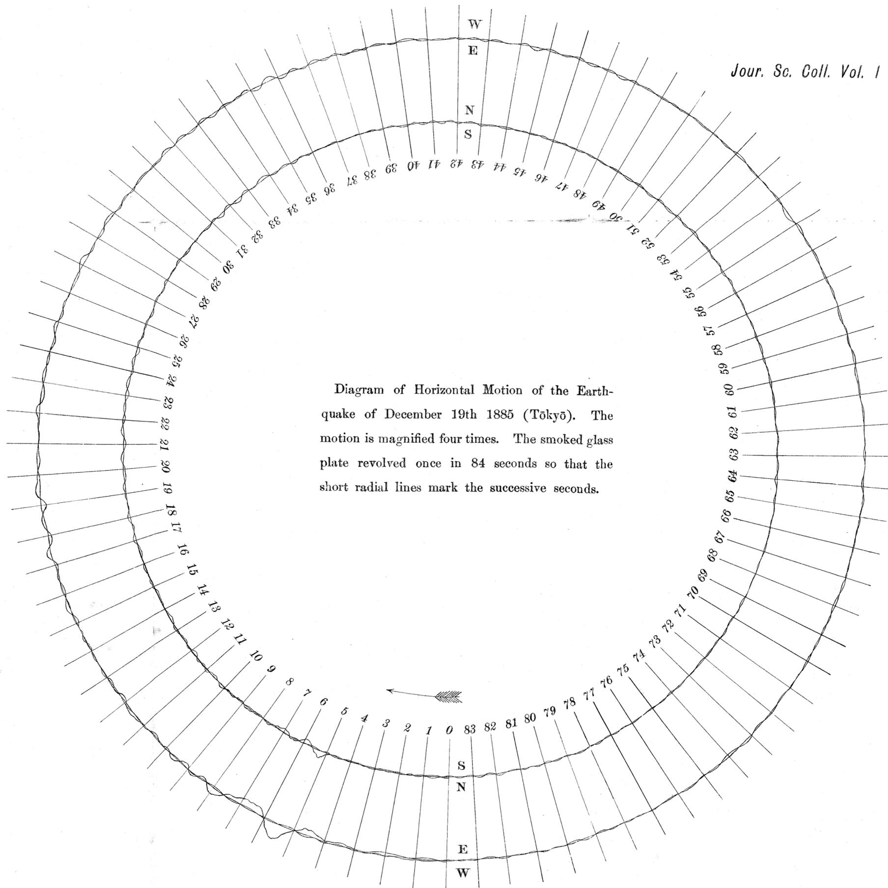
Diagram of Horizontal Motion of the Earthquake of December 19th 1885 (Tōkyō). The motion is magnified four times. The smoked glass plate revolved once in 84 seconds so that the short radial lines mark the successive seconds.
