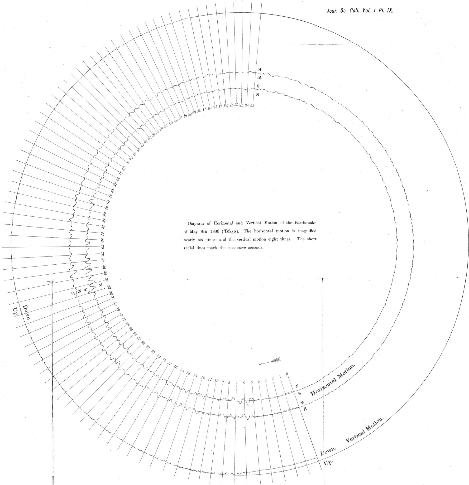
Diagram of Horizontal and Vertical Motion of the Earthquake of May 8th 1886 (Tōkyō). The horizontal motion is magnified nearly six times and the vertical motion eight times. The short radial lines mark the successive seconds.
