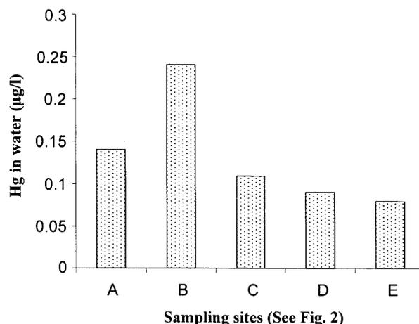
Fig. 5. Mercury content in water from the Totok River and the Buyat River.
