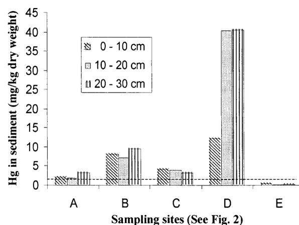
Fig. 6. Mercury content in sediment from the Totok River and the Buyat River.
