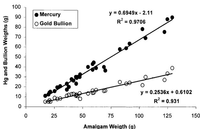
Fig. 4. Relation between recapture mercury (●); gold bullion (○) and amalgam weight.
