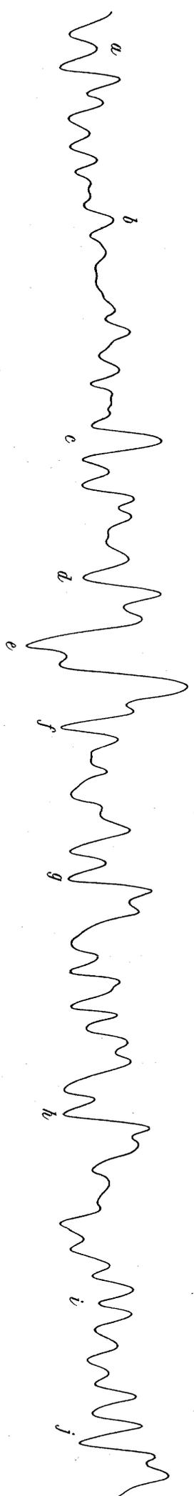
Fig. 12. Lateral and Vertical Vibrations of the Carriage "Goryo-sha."
