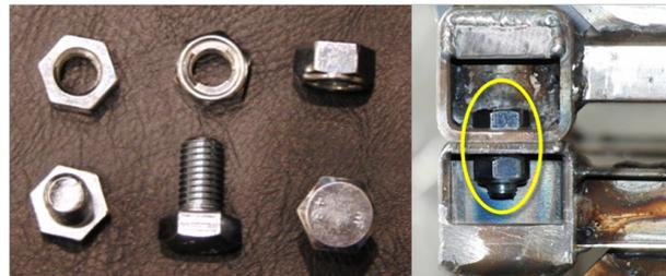
Figure 6.2: Detail of the bolts used to emulate twistlock (left), and disposition of the bolts in the system (right).
