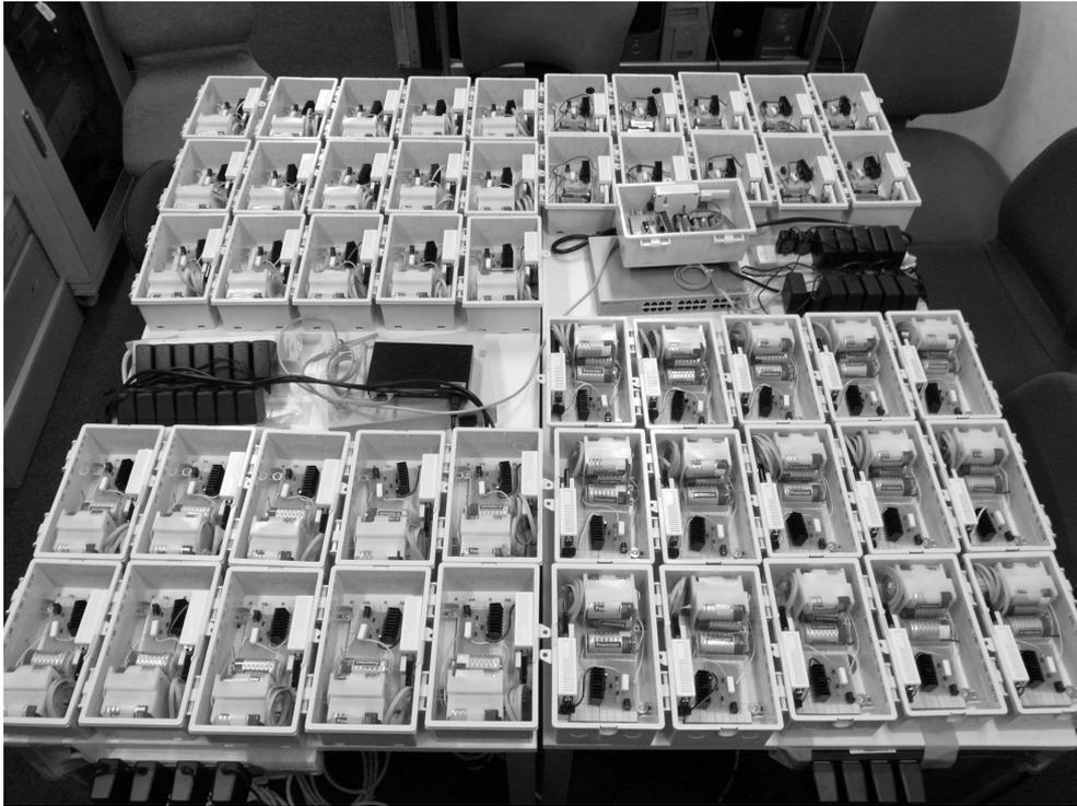
Figure 5.1: UTMESH overview: 51 wireless nodes gathered at the laboratory, in Eng. Bldg. 2 at the University of Tokyo.
