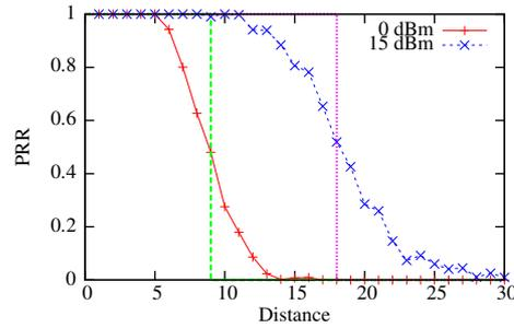
FIGURE 4.1: The packet reception ratio (PRR) vs. the distance between two MICA2 motes under various transmission powers.
