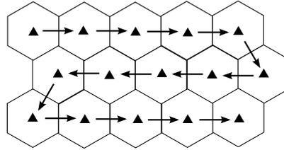
FIGURE 4.4: The optimal movement schedule of the mobile anchor when no information about sensors' positions is available. The triangles represent the way points of the mobile anchor. The edge length of each hexagon is  $r_d$ .
