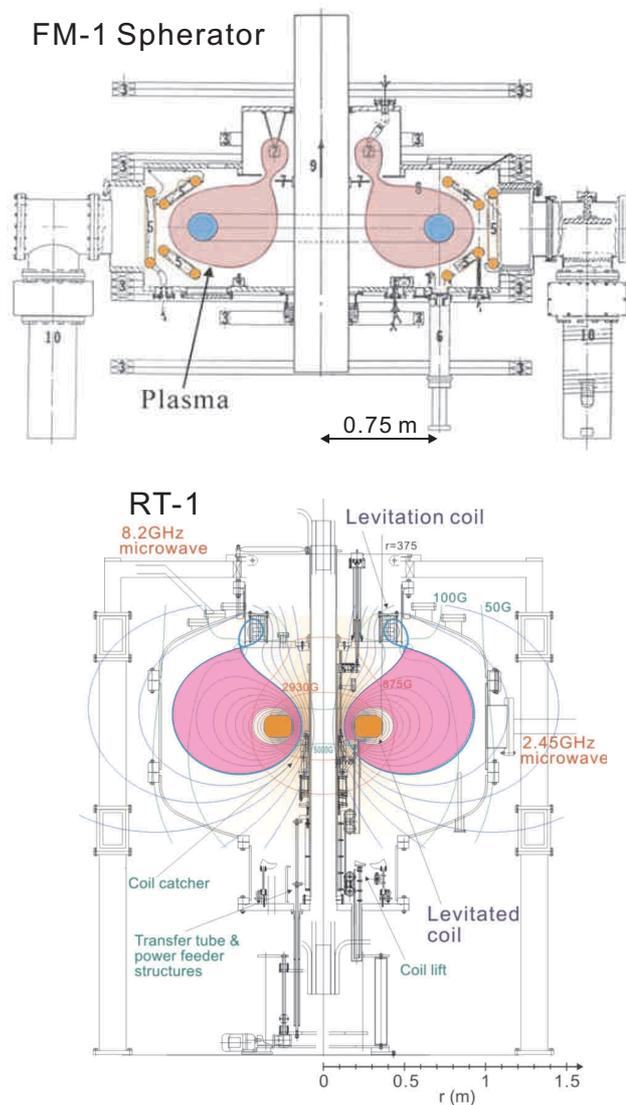
Figure 2.1: Comparison drawing of the magnetic field configurations of FM-1 Spherator and RT-1. Because the floating magnet in FM-1 Spherator was unstable to tilting direction, unlike that of RT-1, there're tilt stabilizing coils in FM-1 [after Ogawa (2009) [67]].
