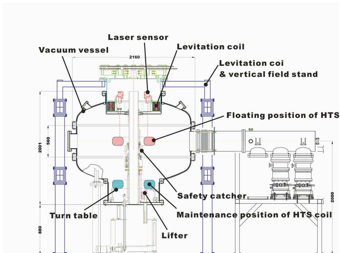
Figure 2.7: Schematic view of the dipole plasma confinement device RT-1. This device is able to generate a plasma with the superconducting internal conductor which is magnetically levitated by the lifting coil.
