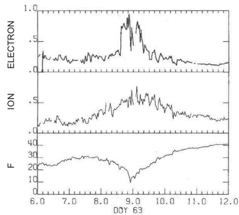
Figure 2.3: Typical observation example of the Jovian plasma. Shown are electron densities and the nominal ion densities and the field strength  $F$ . The field strength decreases at the time of maximum particle densities. This field depression is due to the plasma diamagnetic effect [after Bridge (1979) [21]].
