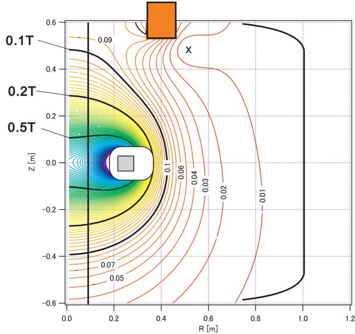
Figure 2.11: Magnetic field strength of the RT-1 configuration. When the F-coil is levitating: separatrix configuration. The unit is given in tesla.
