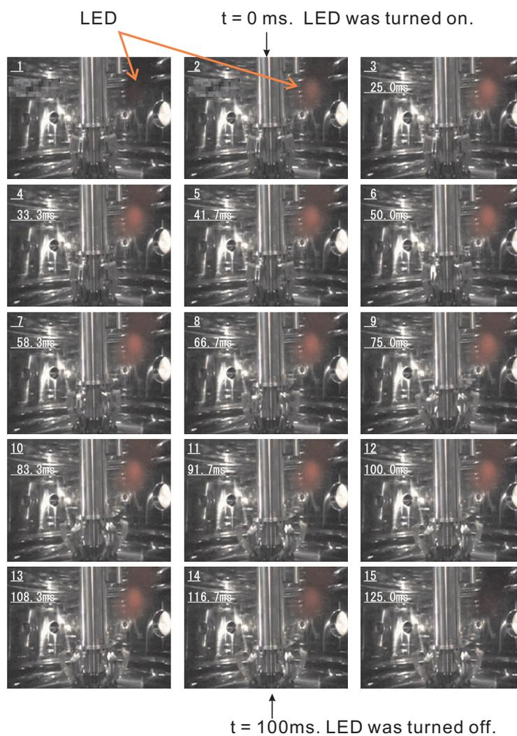
Figure 2.14: A sequence of photographs of the opening of the safety catcher. The pulse duration of the red-colored LED is set to 100 ms. The catcher certainly opens in 100 ms.
