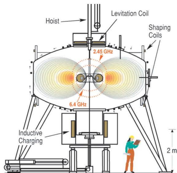
Figure 2.5: Schematic drawing of the LDX device [after Garnier (2006) [57]]. The chamber radius is about 2.5 m and the volume of the plasma is designed large to obtain the stabilization effect of the plasma compressibility.
