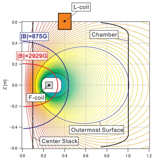
Figure 2.9: Magnetic field configuration of RT-1. When the L-coil current is turned off: pure dipole configuration. The magnetic field is exactly symmetrical about the mid-plane.
