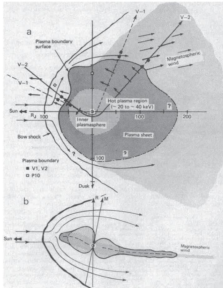
Figure 2.2: Plasma model of the Jovian magnetosphere in (a) the equatorial and (b) the meridional planes. The model emphasizes the hot plasma regions. Question marks indicate areas of uncertainty. The long arrows indicate solar wind flow direction [after Krimigis (1979) [3]].
