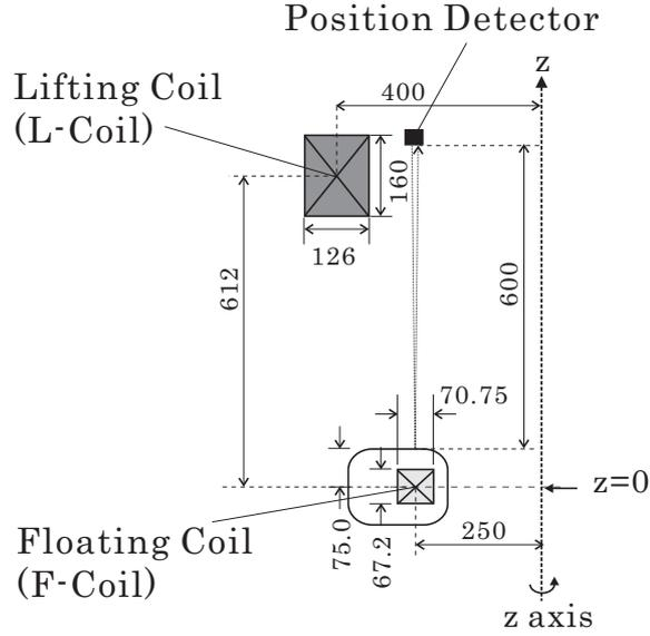
Figure 2.8: The schematic view of the arrangement of the F-coil, the L-coil and the position detectors.
