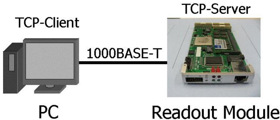
Fig. 8. Measurement setup. The Readout Module and PC, which were connected directly with a crossover cable, acted as the TCP server and client, respectively.
