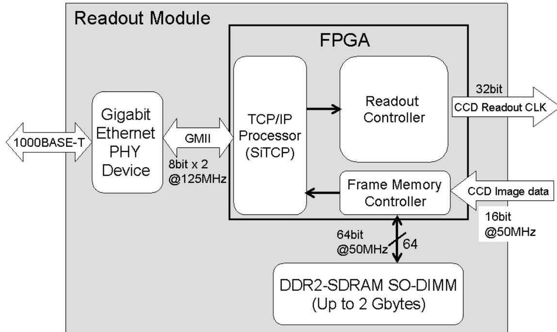
Fig. 6. Block diagram of the readout module
