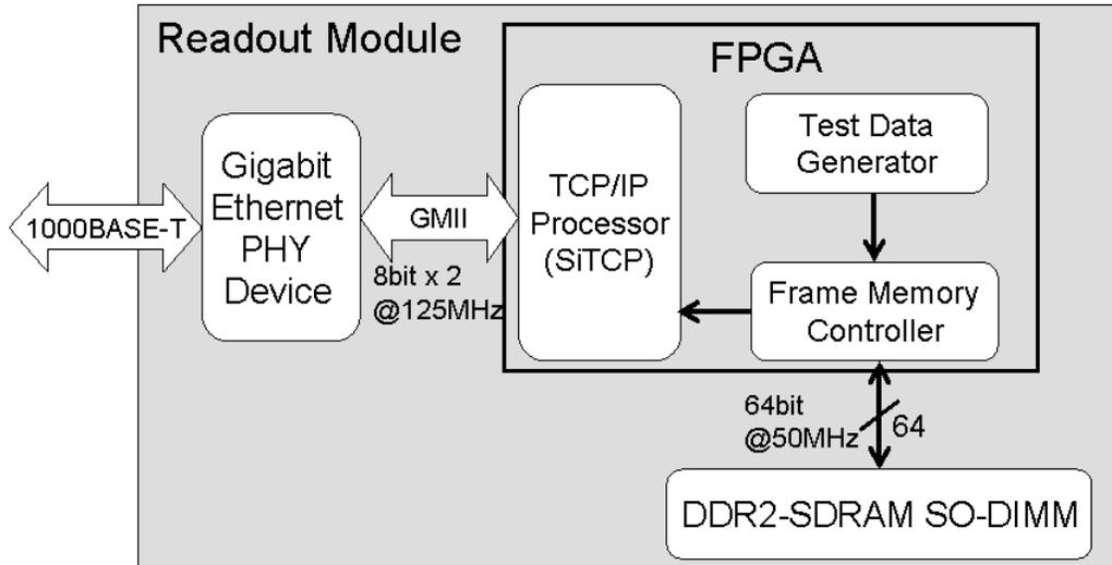
Fig. 7. Block diagram of the test circuit
