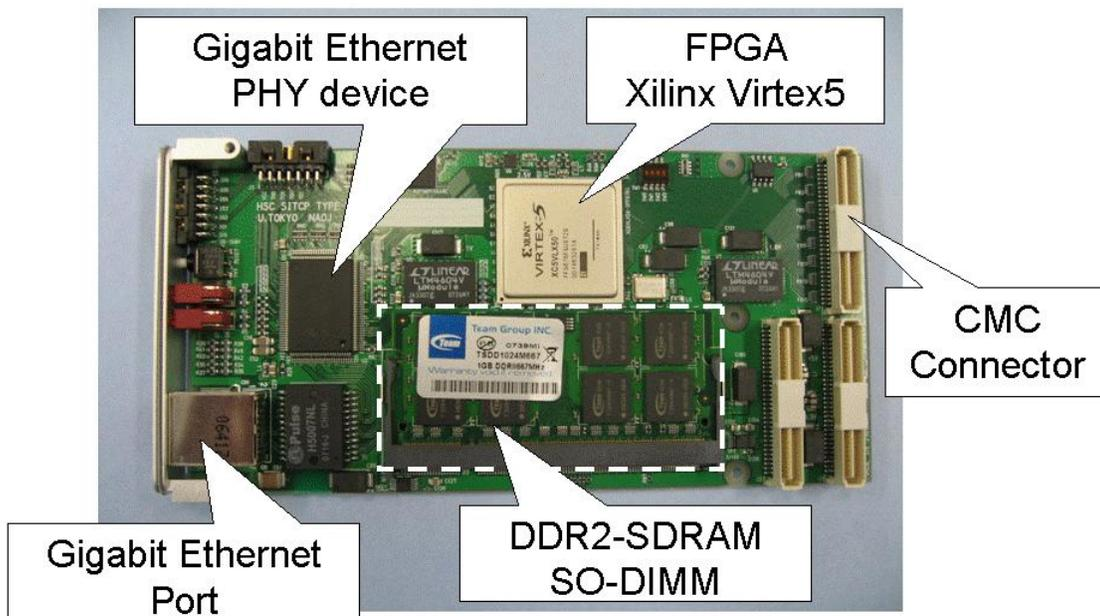
Fig. 5. Photograph of the prototype readout module (Top view)
