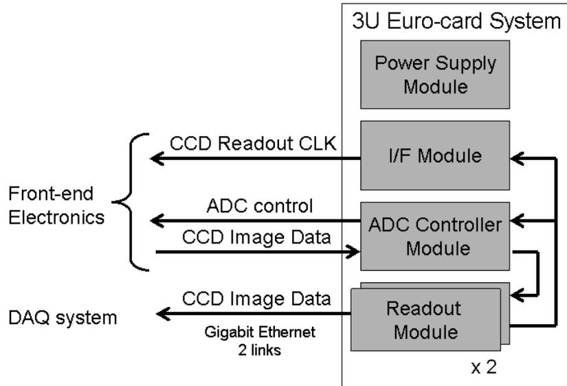
Fig. 3. Schematic diagram of a planned back-end electronics system
