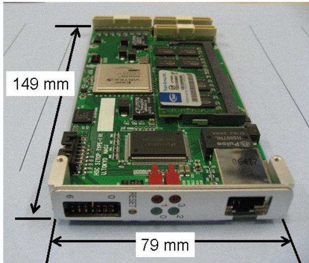
Fig. 4 Photograph of the prototype readout module (Front view)
