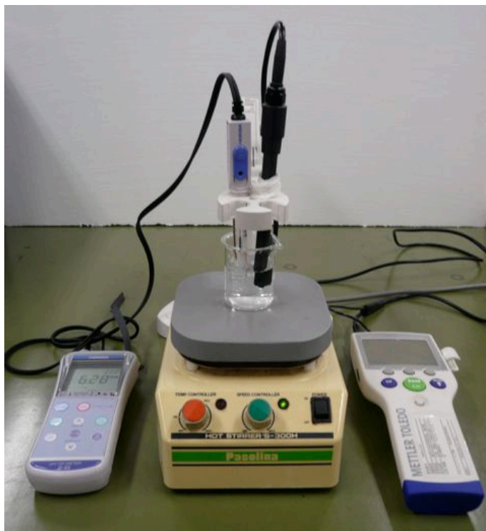
Figure 3.3: Measurement of DO concentration and pH.
