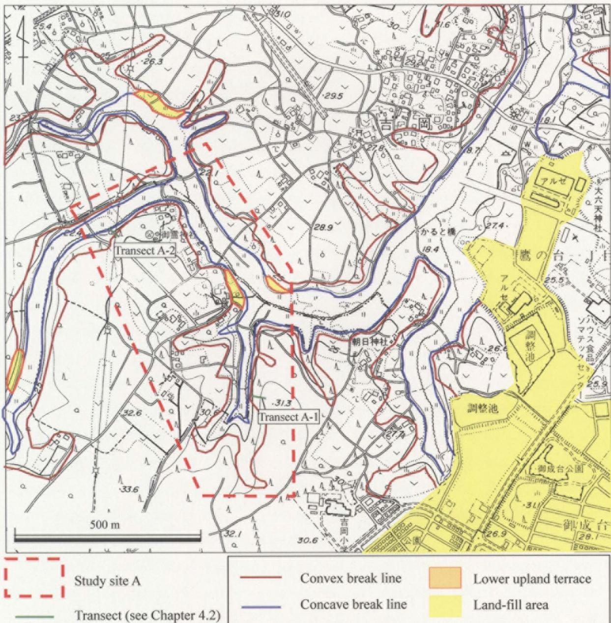
Figure 3.1-3 Detailed-scale land-form classification is Site A.
