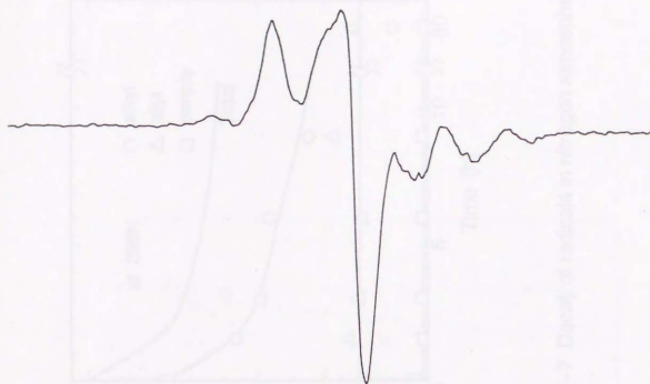
Fig.2-4 ESR spectra of porous polyethylene irradiated by gamma-ray in air
