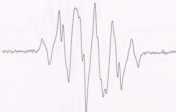
Fig.2-1 ESR spectra of porous polyethylene irradiated in nitrogen atmosphere
