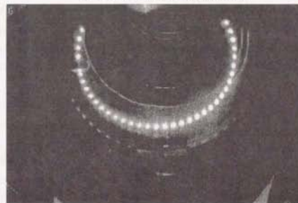
Figure 4.9: Improvement of the beam spot distortion with a beam profile which provides the beam waist in the middle of two mirrors, and correspondent simulation
