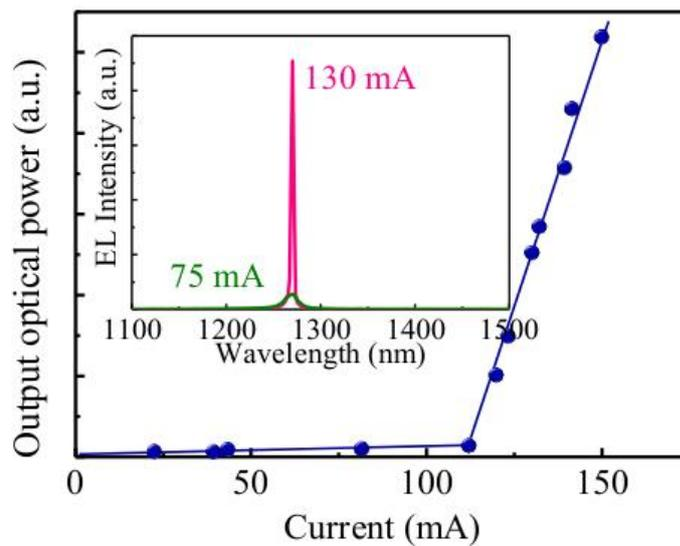
**Figure 3.** Room-temperature light-current characteristics and (inset) electroluminescence spectra of the broad-area InAs/GaAs QD laser on SOI substrate fabricated by metal-stripe wafer bonding.
