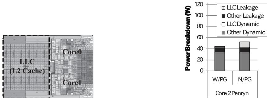
Figure 1.2: The area of the LLC in a commercial mobile processor and the power breakdown of the processor (remade from Figure 4 in V. George *et al.*(2007) [2] and Figure 1 in S. Li *et al.*(2011) [3] respectively)
