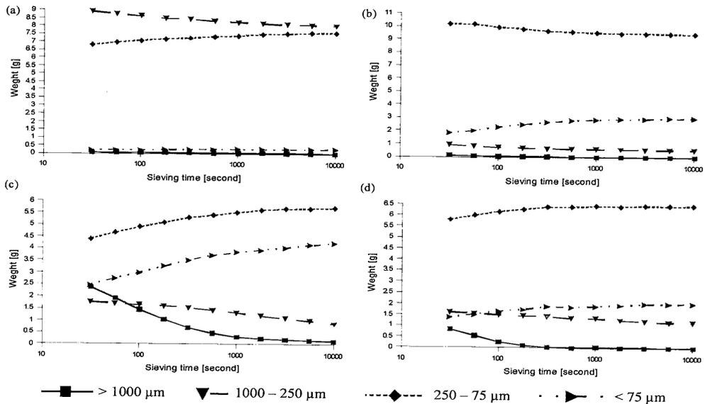
**Figure 2.** Time series of the soil weight on each sieve in a preliminary test of dry-sieving of (a) dune sand (sample no. 19), (b) castanozem (no. 2), (c) chernozem (no.3) and (d) loess (no. 12).
