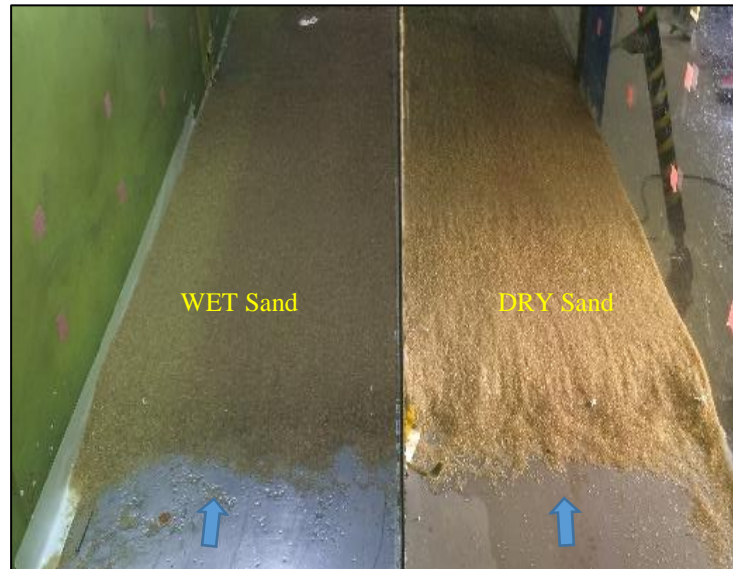
Figure 5.19 Almost similar appearance in WD and DD for high \Delta H . No air escaping mark left (R14)
