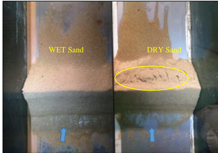
Figure 5.18 Air in void is significant for low \Delta H . Many air escaping marks left on back dune (R2)
