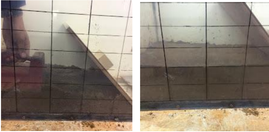
Figure 4.8: Tamping of base layer soil.
