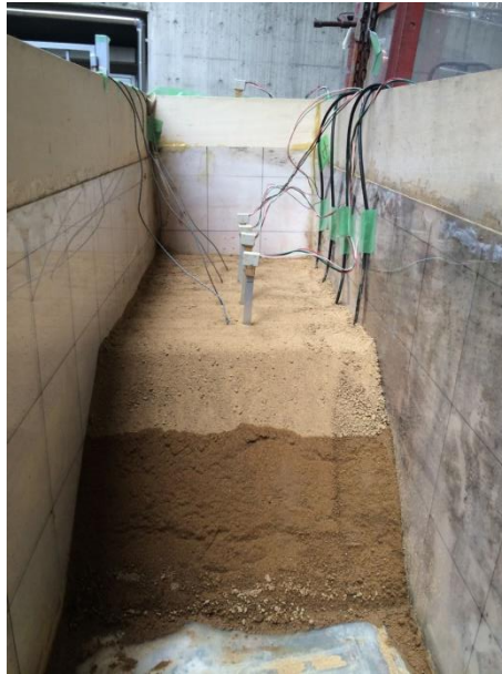
Figure 4.5: Installation of sensors s after slope completion.
