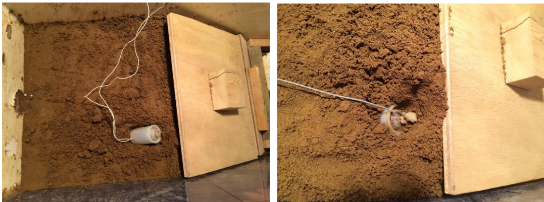
Figure 4.9: Installation of solenoid and wave sensor.
