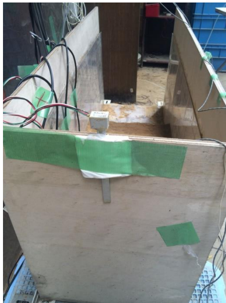
Figures 4.6: Reference tilt sensor attached to the wall.
