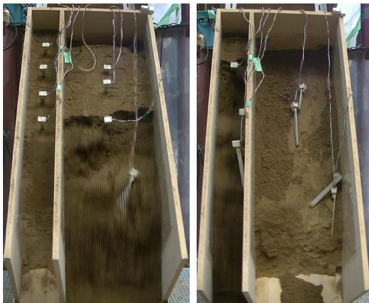
Figure 4.19: Failure of 10 and 25 cm-wide cells.
