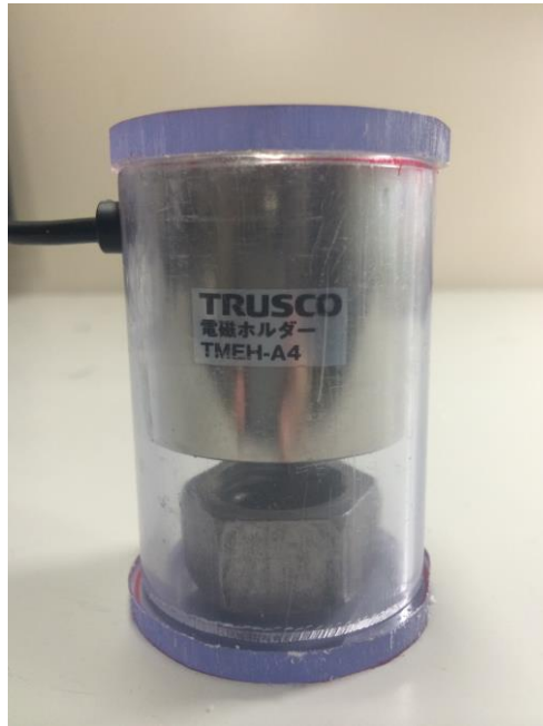
Figure 8.23: solenoid used for large scale model test.
