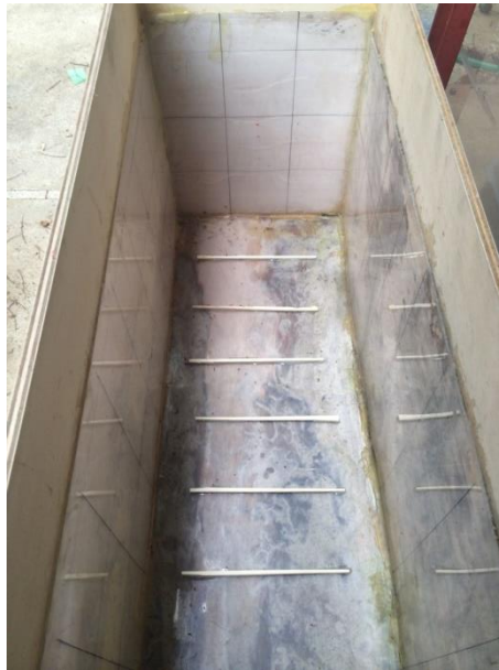
Figure 4.3: Wooden strips fixed at the bottom of tank to increase the friction between soil and the tank to prevent failure occurring from the bottom interface.
