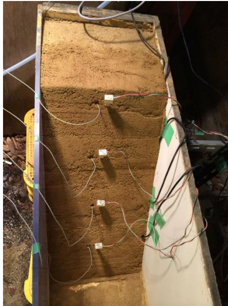
Figure 4.13: Installation of sensors s after slope completion.
