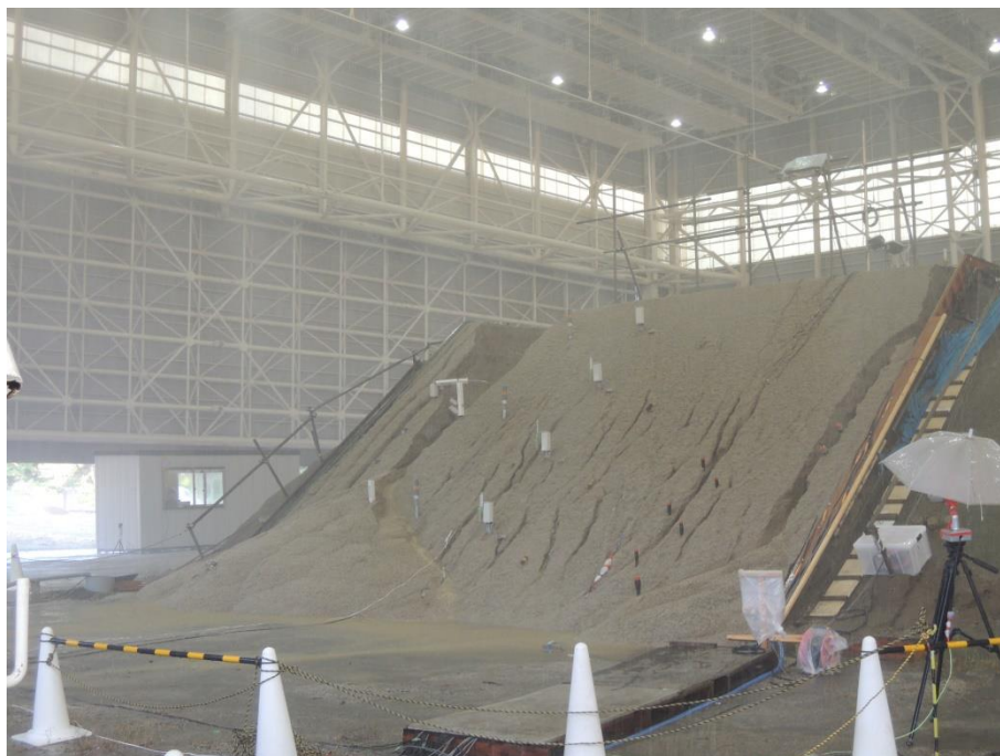
Figure 8.30: Wave receivers removed due to collapse of slope surface caused by runoff erosion.
