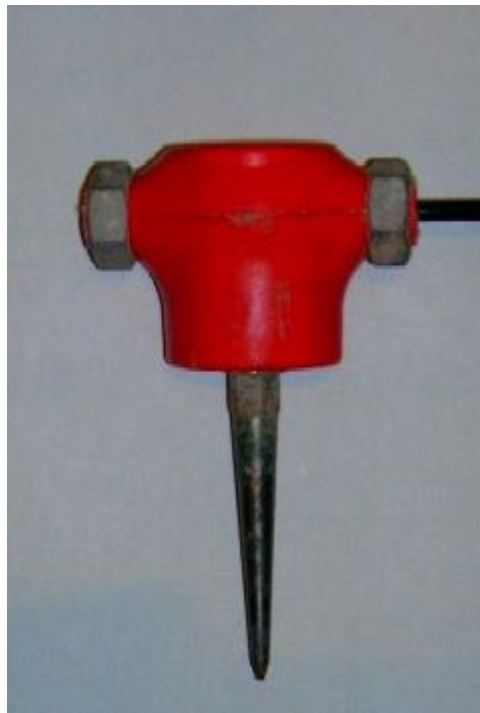
Figure 8.22: Geophone acting as wave sensor.
