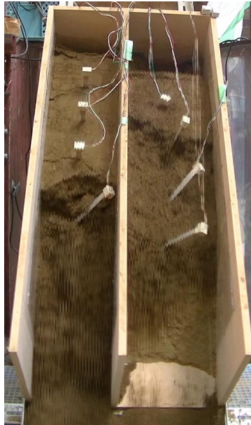
Figure 4.18: Failure of 15 and 20 cm-wide cells.
