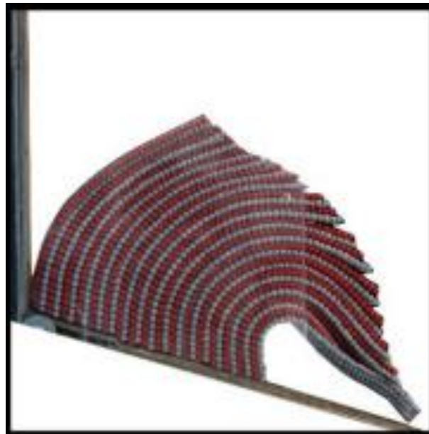
Figure 5.16: deformational of slope using discrete element method (Chuang 2014).
