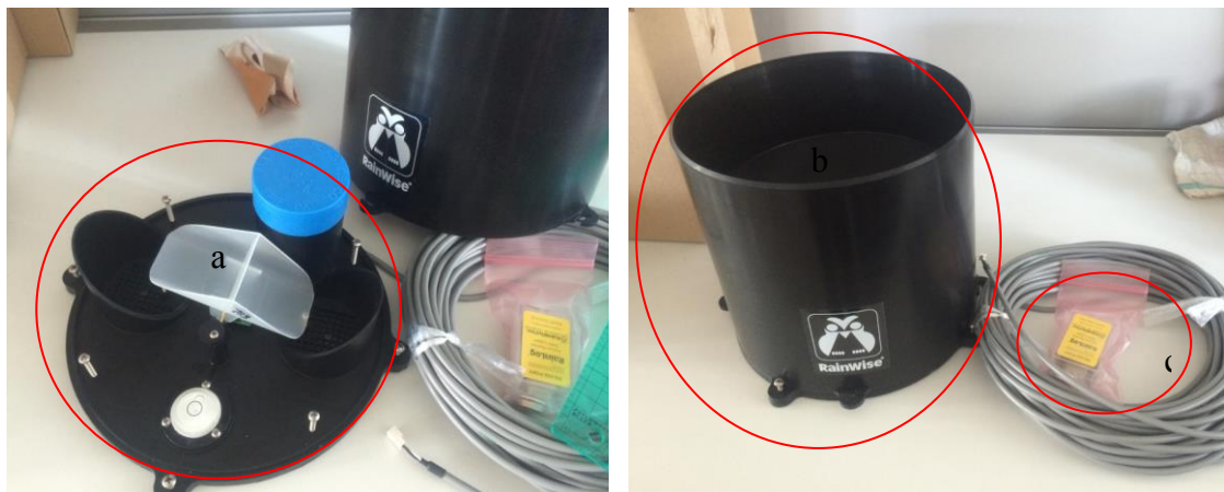
Figure 13 - Rain Gauge With Tipping Bucket (a), 8" Diameter Collector (b) and auto logger (c)
