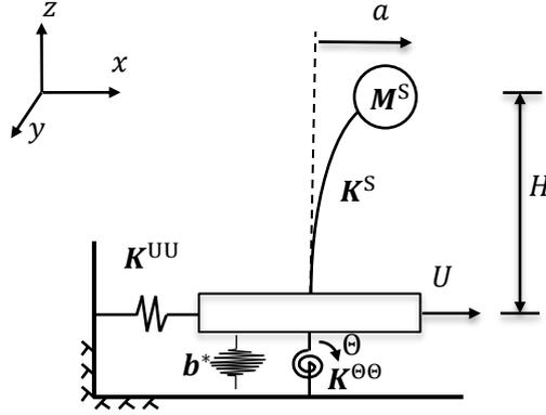
Figure 5.1: Conventional mass-spring soil spring model
