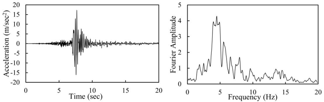
Figure 6.4: Input ground motion GM2 in time and frequency domains
