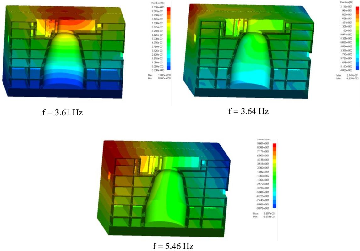
Figure 7.3: The three dynamic modes for the structure used
