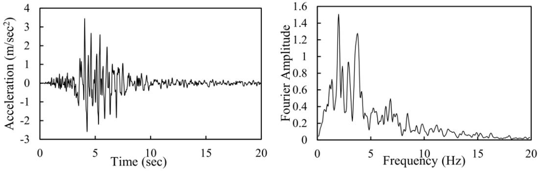
Figure 6.3: Input ground motion GM1 in time and frequency domains
