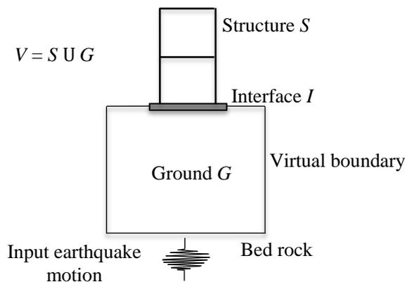
Figure 3.1: Analysis domain for the seismic response analysis considering SSI
