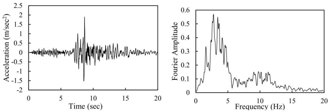
Figure 6.5: Input ground motion GM3 in time and frequency domains
