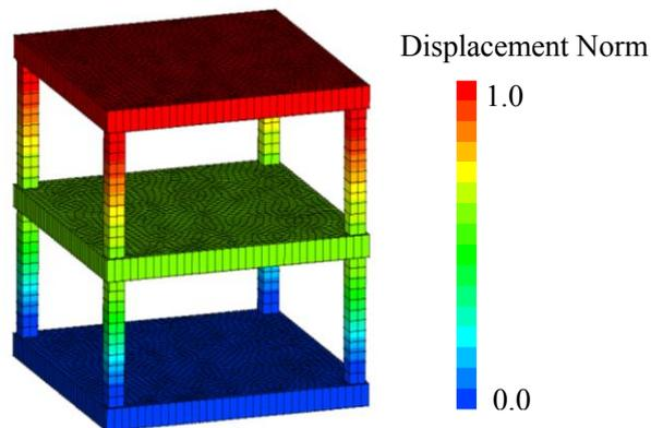
Figure 6.6: Minimum natural frequency of the structure = 1.84 Hz
