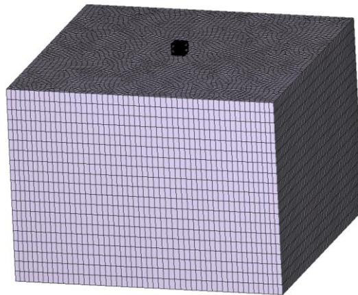
Figure 6.1: Two storey building with the soil domain considered
