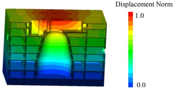
Figure 6.12: Minimum natural frequency of the structure = 3.80 Hz
