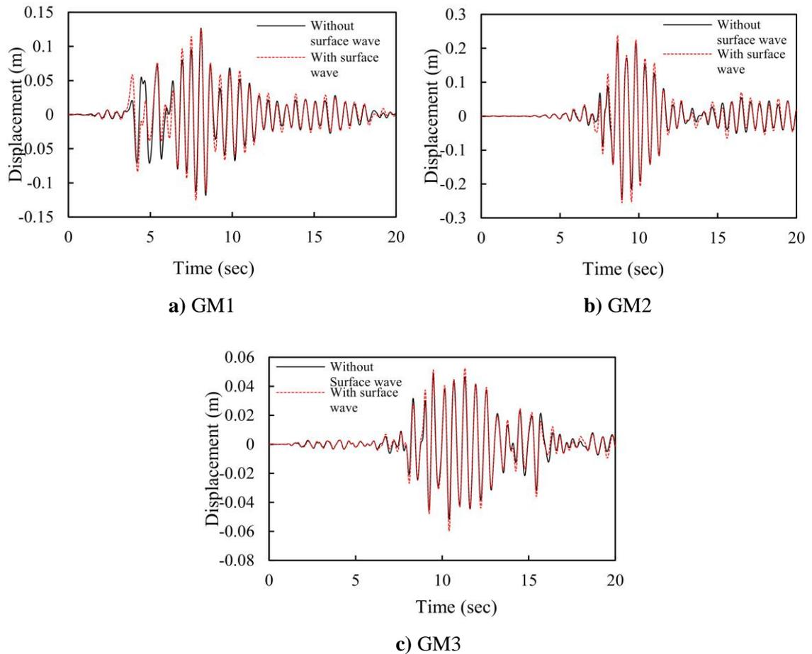
Figure 6.9: Comparison of x-direction displacement response at the top of structure for mass spring system with and without inclusion of surface wave
