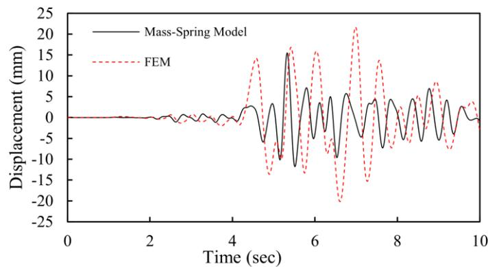
Figure 6.13: Comparison of  $x$ -direction displacement response at the top of structure obtained from mass spring model and FEM without the inclusion of surface wave
