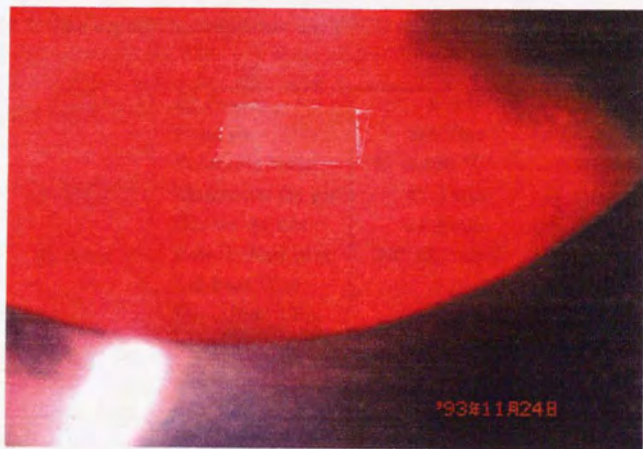
Figure 4.21: A photograph during YBCO large-area deposition on YSZ substrate.
