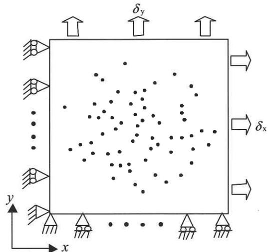
Fig. 3 Perforated sheet under uni/biaxial tension
