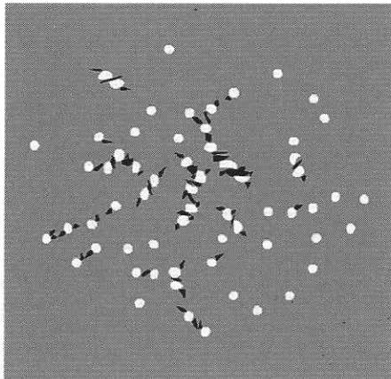
Fig.11 Void linking (biaxial loading,  $\delta_x = \delta_y = 7.615\text{ mm}$ )
