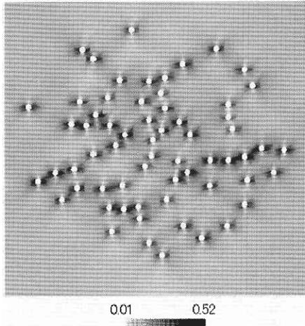
Fig. 5 Equivalent strain (uniaxial loading)
