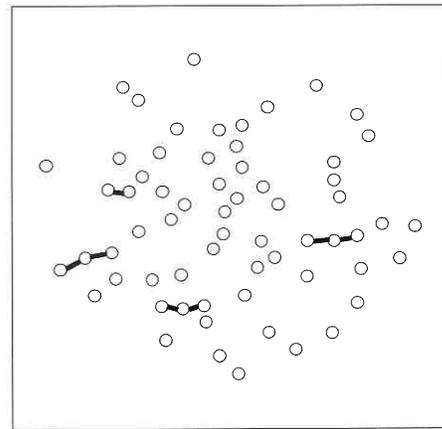
Fig. 8 Experimental void linking (uniaxial loading)
