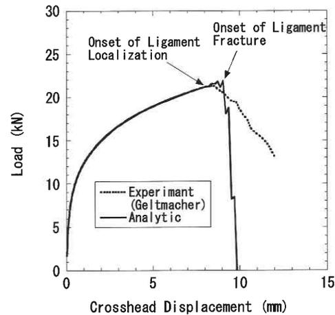
Fig. 6 Load-displacement curves (uniaxial loading)
