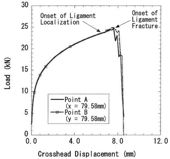
Fig. 10 Load-displacement curve (biaxial loading)
