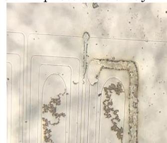
Figure 2 Damaged grid due to sparks
