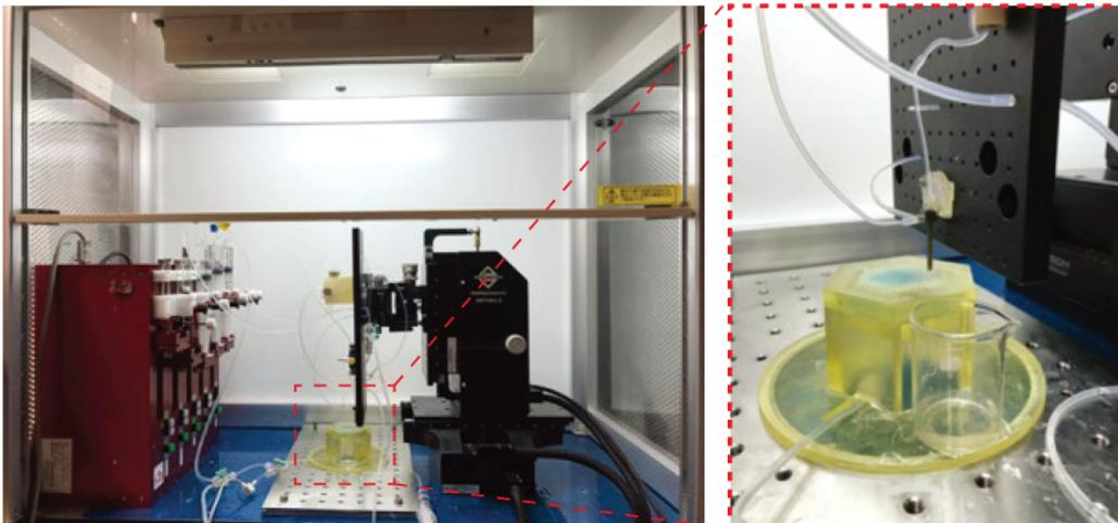
Fig. 2 Schematic and actual photo of the bioprinter for cell fiber printing.
