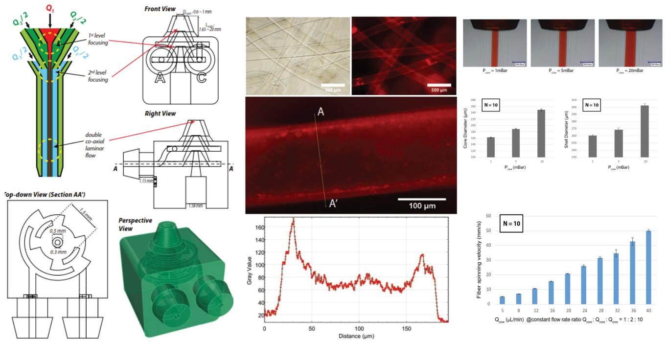
Fig. 3 Design and tests of the printhead.
