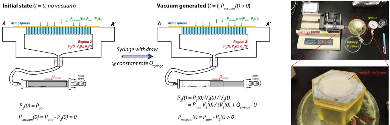
Fig. 4 Design and tests of the syringe-vacuum substrate.
