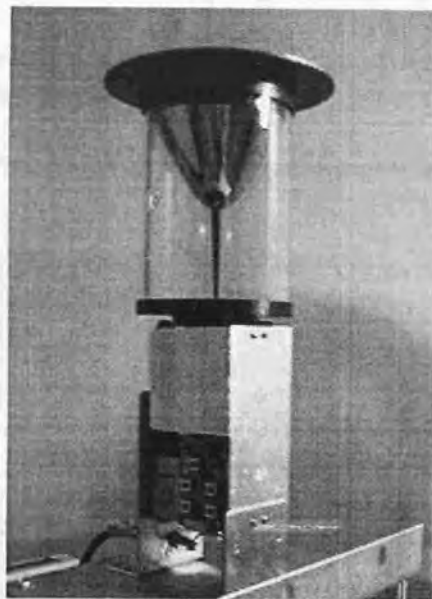
Figure 5.1 Omnidirectional vision sensor.
