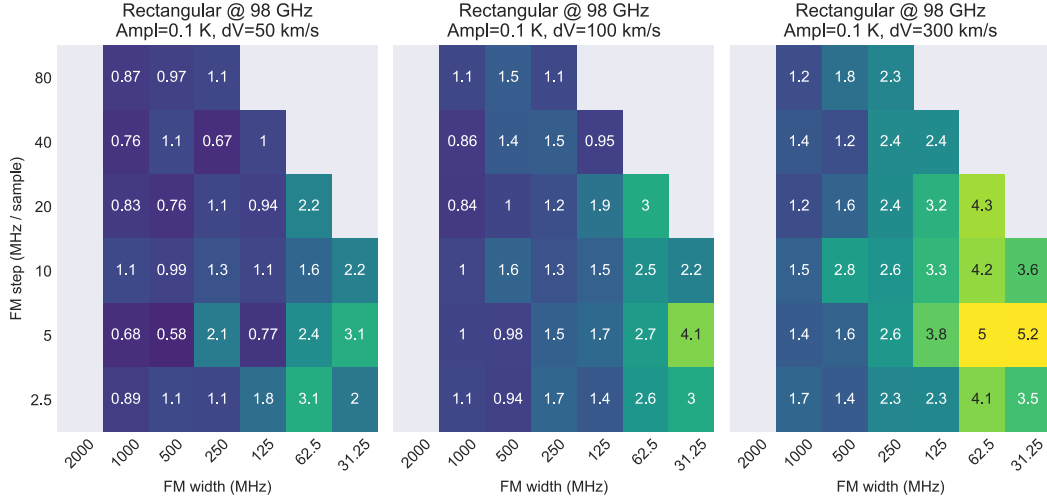
Figure A.16: Heatmaps of reduced \chi^2 after subtracting correlated components at the first iteration between reproduced and model spectra of rectangular models ( \Delta v = 50, 100, 300 km/s from left to right, T_{\text{peak}} = 0.1 K at 98.0 GHz) calculated for various FMPs. The parameters used for calculating reduced \chi^2 are same as figure A.14.
