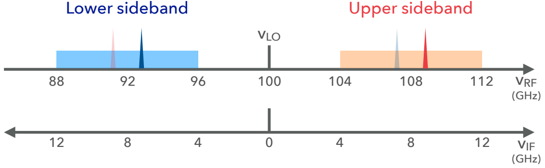
Figure 1.2: Schematic diagram of sidebands in a heterodyne receiver. Once observer configures an LO frequency, then IF frequency is generated like a bottom number line. If observable IF ranges are represented as lightblue and orange boxes, they are called lower sideband (LSB) and upper sideband (USB). Observable IF ranges are constrained by frequency response of a mixer, LNA for IF signal, and also specifications of a spectrometer. The blue and red spike represents spectral lines located at that observed frequencies. The ones of light color represents lines contaminated from each image sideband.
