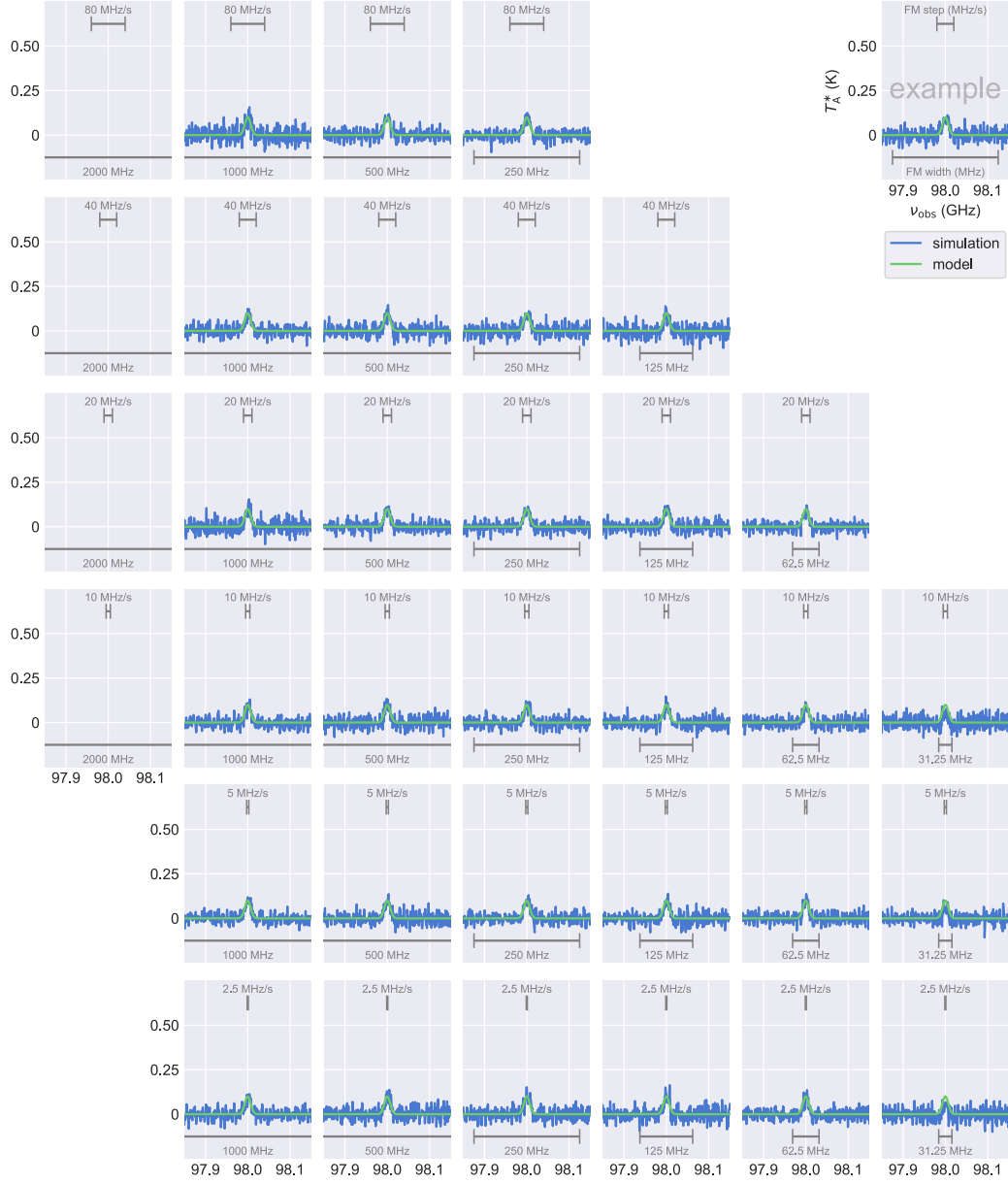
Figure A.4: Grid view of all the results of spectral line simulations with a Gaussian model ( \Delta v = 50 km/s, T_{\text{peak}} = 0.1 K at 98.0 GHz) embedded to timestreams of blank sky observed with various FMPs. Blue and green lines show the reproduced spectrum after signal processing and the model spectrum itself, respectively. Gray bars at top and bottom of a panel indicate an FM step (MHz/sample; printed as MHz/s) and FM width (MHz) of an FMP used for an FMLO observation.
