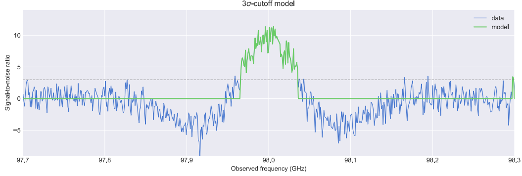
Figure 4.7: An example of the n\sigma -cutoff method, where a spectrum from an FMLO observation and a model as a result of 3\sigma -cutoff (i.e., \theta_{\text{cutoff}} = 3 ) are expressed as blue and green lines. The estimated 1\sigma noise level is indicated as a gray line. The negative sidelobe features at the both sides of a line are artificial ones due to improper estimate of correlated component removal and thus should not be modeled as signals. The n\sigma -cutoff can eliminate such features well, however, faint outer skirts between 0 to 3\sigma are not modeled. We demonstrate that such faint features are also successfully reproduced in after several iterative processes in § 5.3.4.
