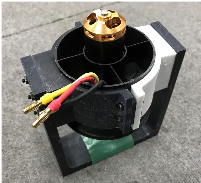
Fig. 4.10: The thrust testbed
