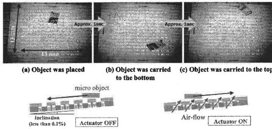
Fig. 4: Micro conveyance experiment of 1 D motion
