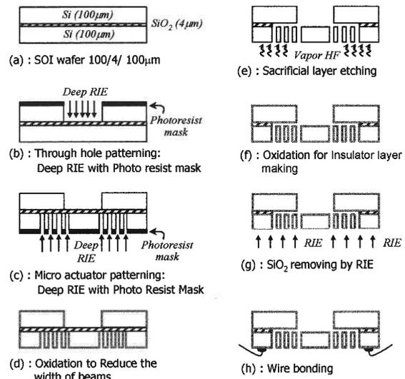
Fig. 5: Fabrication process steps of MEMS actuator
