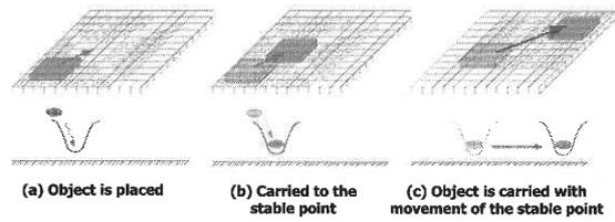
Fig. 12: Concept of micro conveyance by many cells
