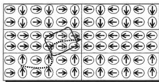
Fig. 7: MEMS actuator distributed structure
