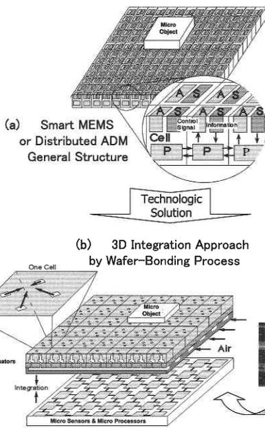
Fig. 11: Smart MEMS design approach
