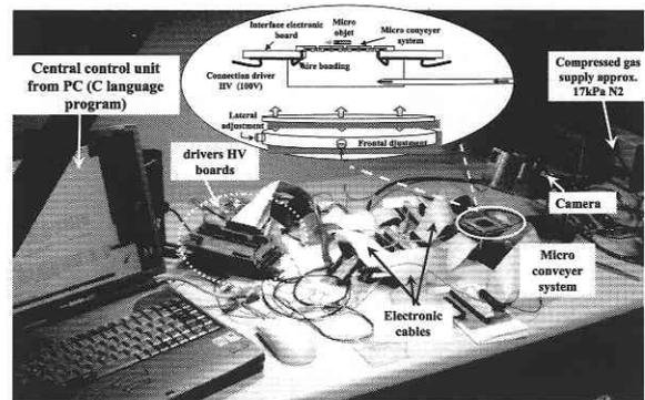
Fig. 9: Test bench of the micro conveyance system
