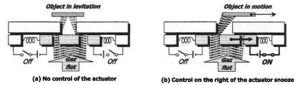
Fig. 3: Principle of the air-flow micro actuator.
