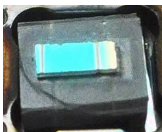
Fig. 4.4 sample picture of a BaTiO 3 film grown on a Ge substrate at an oxygen background pressure of 2 \times 10^{-5} Torr at 600 °C.
