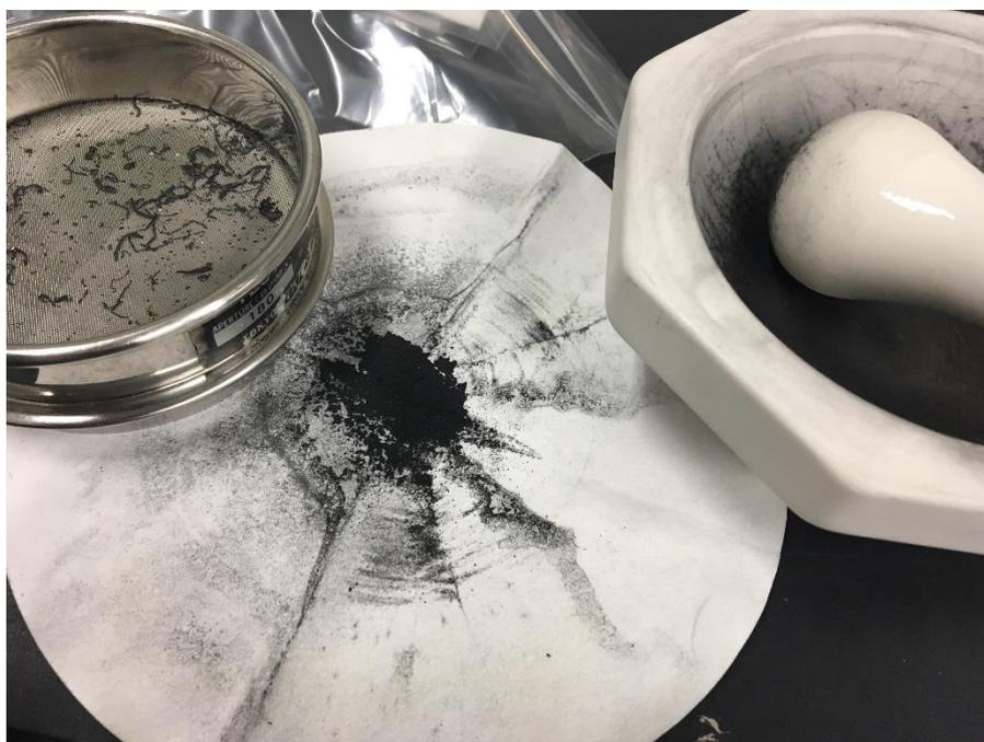
**Figure 5-8.** Larger particles in 180 $\mu$ m sieve (left), separated powder sample for XRD analysis (middle) and the mortar (right)
