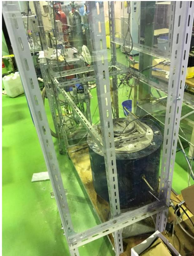
**Figure 2-16.** The protective shield of the salt bath
