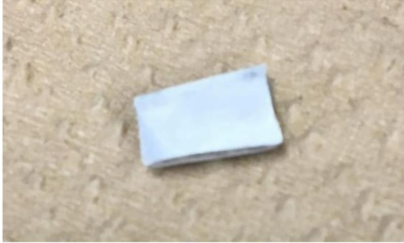
**Figure 4-6.** Stainless plate after acid dissolving
