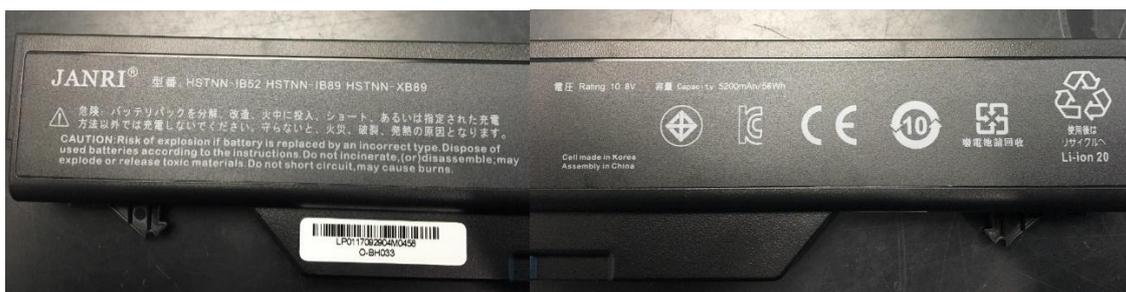
Figure 2-3. The Li-ion battery pack used in the research
