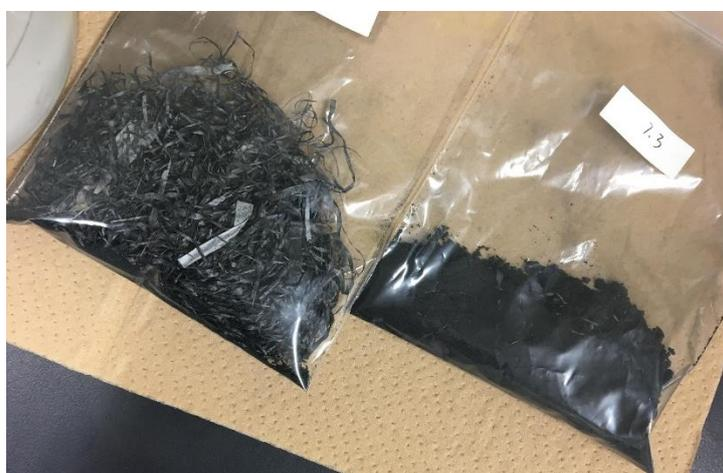
**Figure 2-8.** Ribbon (left) and powder (right) LIB sample
