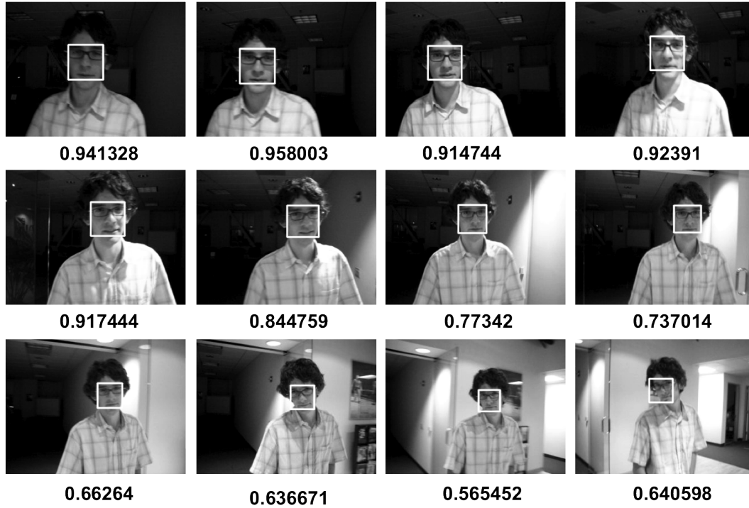
Figure 3.3: Experiment on tracking with size feature. The size value of each object state is shown under the frame of image.
