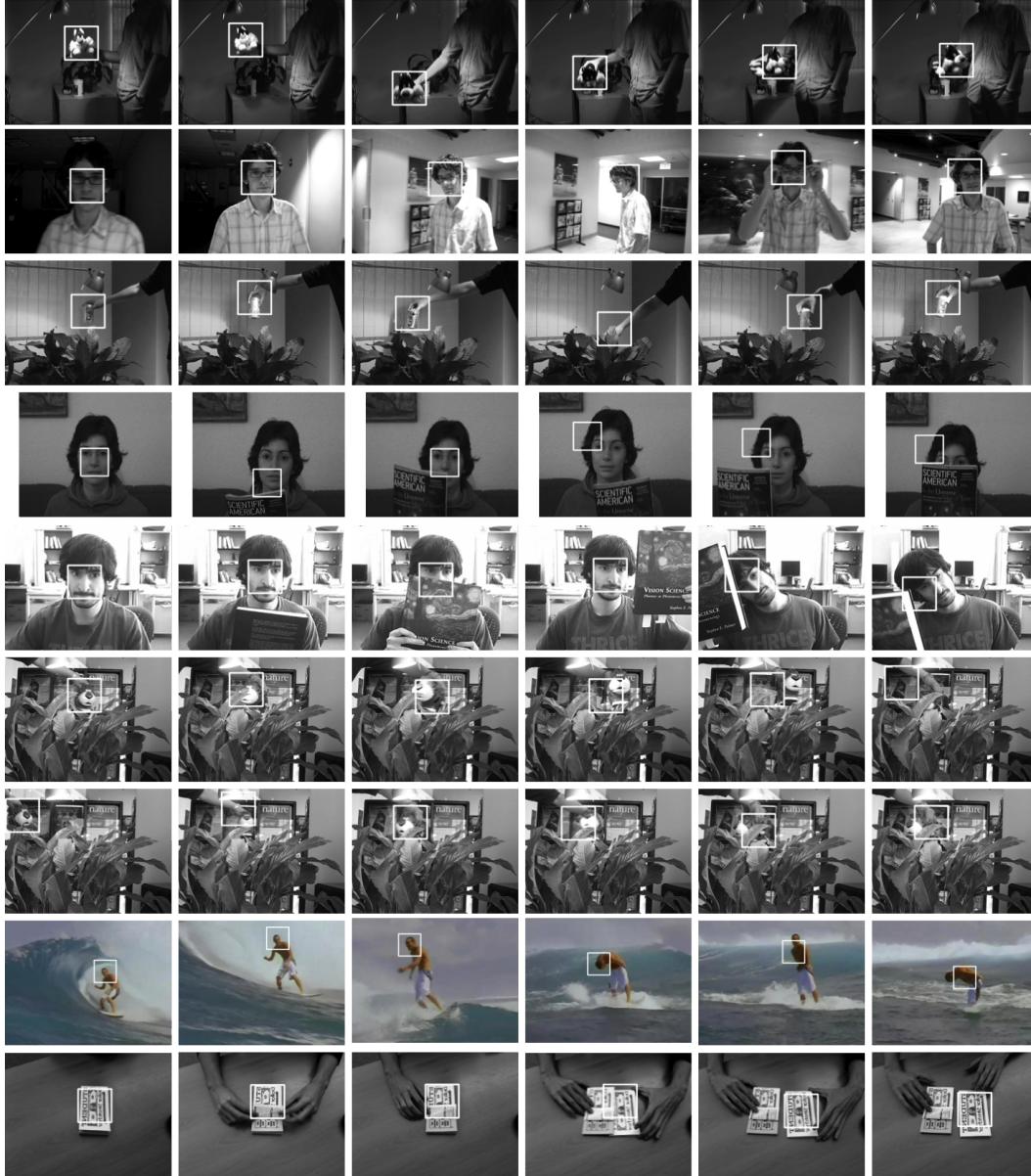
Figure 2.12: Tracking results from software simulation. Video sequences from top to bottom: Sylvester, David Indoor, Cola Can, Occluded Face, Occluded Face 2, Tiger 1, Tiger 2, Surfer, Coupon Book.
