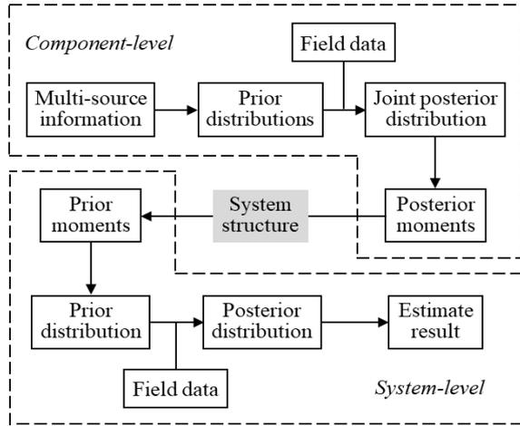
Figure 1. Procedure of system reliability evaluation
