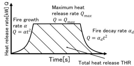
Figure.1 Modeling of a heat release curve
