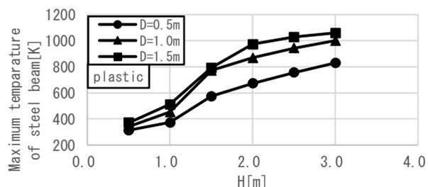
Figure.6 Height and Bottom length of combustibles – steel beams maximum temperatures relationships (plastic combustibles)
