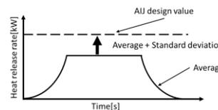
Figure.9 Concept of design heat release rate
