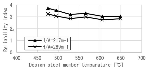
Figure.12 Reliability index  $\beta$ -design steel beam temperature relationships (plastic)
