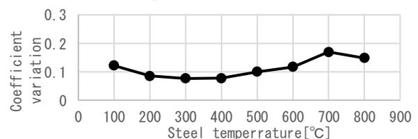
Figure.10 Coefficient variation of steel strength at high temperature
