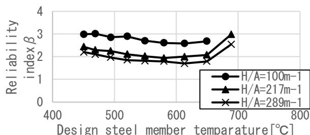
Figure.11 Reliability index  $\beta$ -design steel beam temperature relationships (wood)
