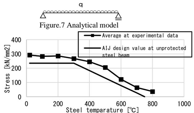
Figure.8 Steel strength at high temperatures
