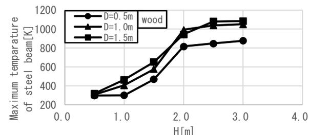
Figure.5 Height and bottom length of combustibles – steel beams maximum temperatures relationships (woody combustibles)
